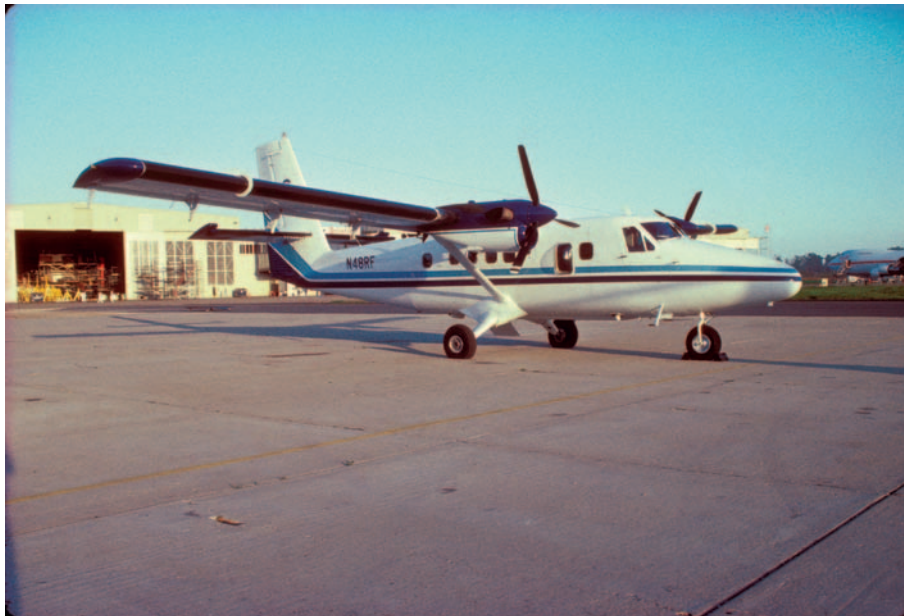
Figure 4 NOAA Twin Otter survey aircraft with bubble window (under propeller) and belly window port (above tire) (Photo: K. Forney).
