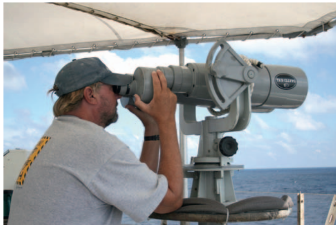
Figure 2 "Big eyes" used to search for marine mammals on large survey vessels. (Photo courtesy of Protected Resources Division, Southwest Fisheries Science Center, NOAA).
