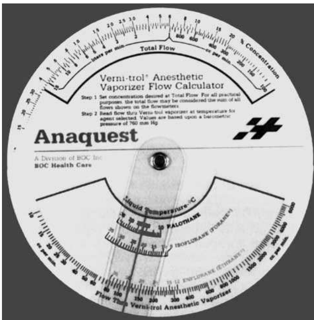
Figure 5-3 Circular slide rule for calculation of oxygen flows for an anesthetic machine with a measured-flow VOC vaporizer (Verni-trol, Copper Kettle). The rule can be used for multiple anesthetic agents and a variety of total oxygen flow rates over a range of temperatures. Calculations can be made according to the following equations (using halothane as the anesthetic agent):
