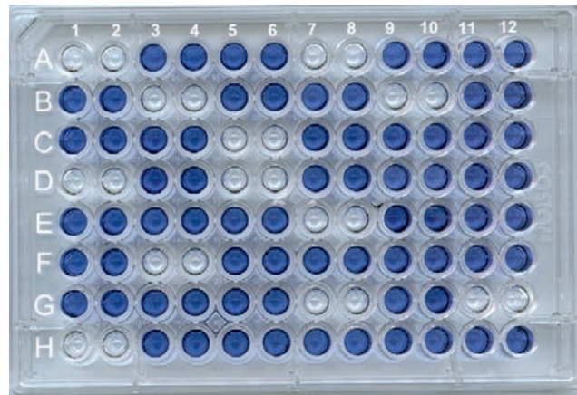
FIGURE 5.10 Competitive enzyme-linked immunosorbent assay (cELISA) for caprine arthritis encephalitis viral (CAEV) antibodies. Undiluted serum samples in duplicate are added to antigen-coated wells of a commercial cELISA test for CAEV antibodies. After removal of the test sera, an antibody specific for CAEV antigen and coupled to horse-radish peroxidase is added. The detector antibody is removed after incubation, and a substrate is added to detect the presence of bound detector antibody. If there are antibodies specific for CAEV in the test sera, these antibodies bound to antigen will prevent the detector antibody from binding. A positive sample will therefore show less enzyme product (color) than the negative controls. Cut-off values are determined by reading the intensity of the reaction with a spectrophotometer, although visual inspection can usually detect positive samples. Wells A1–2 and G11–12: positive controls; wells B1–2 and H11–12: negative controls; wells D1–2, H1–2, B3–4, F3–4, C5–6, D5–6, A7–8, E7–8, G7–8, and B9–10: samples positive for antibodies to CAEV.
