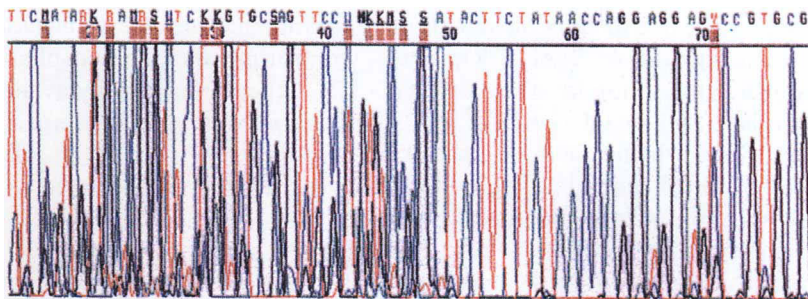
Figure 10.1 Data produced by dye terminator sequencing of primer-dimer contaminated PCR product
