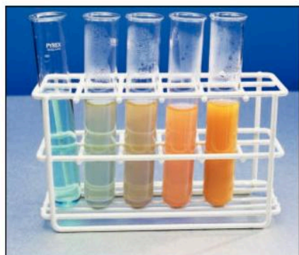
Figure 5.1.1 Testing for reducing sugars. The highest concentration of sugar is on the right.
