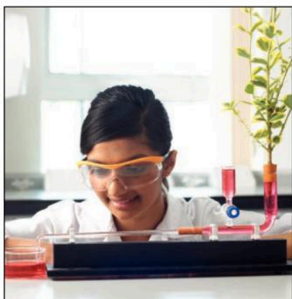
Figure 6.7.1 A potometer for measuring the rate of water uptake by leafy shoots. Figure 1 on page 101 is a diagram of a potometer like this one.
