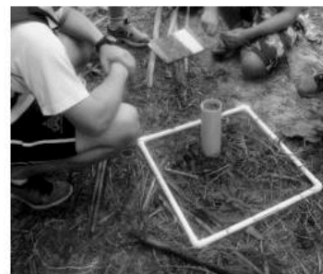
▲ Figure 18.2 Students measuring the infiltration rate – the speed at which a known volume of water enters a known area of soil. They compared the rates for soils in a palm oil plantation with soils in a rainforest
