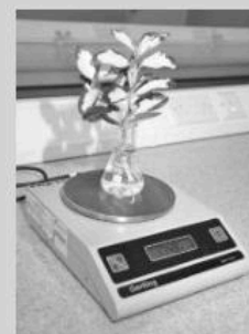
▲ Figure 7.16 A mass potometer
