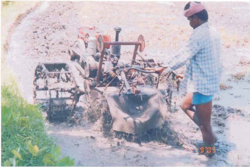
Fig. 15.1 Puddling rice field with power tiller
