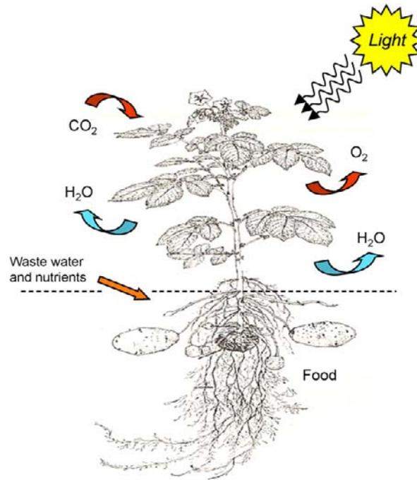
**Figure 17.1: Plants as life support machines for space travel. Plant photosynthesis could provide oxygen and food, while removing carbon dioxide. Plant growing systems could also help waste water processing where the plant transpiration serves as a final distillation step after which the humidity is condensed as clean water.**
