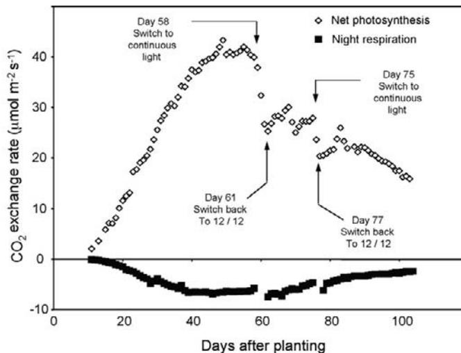
Figure 17.14: Effect of changes in photoperiod on the carbon dioxide exchange rate of a 20 m<sup>2</sup> potato stand. On day 58, the photoperiod was changed from 12-h to 24-h (i.e., continuous light), which resulted in drop in the instantaneous photosynthetic rates. Switching back to 12 h at day 61 allowed photosynthetic rates to slowly increase. A similar effect was observed between days 75 and 77 (source: Wheeler et al., 2008a).
