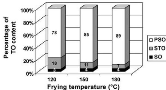
**Figure 11.4:** Average oil fractions absorbed by potato slices during frying at 120, 150, and 180°C. TO: total oil; PSO: penetrated surface oil; SO: surface oil; STO: structural oil (reprinted with permission from *J. Food Eng.*, 2008, 87, 200–212).
