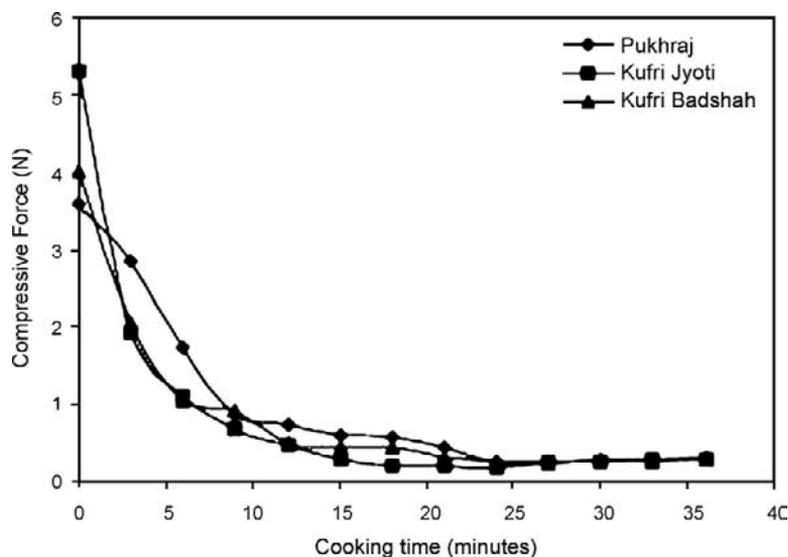
**Figure 9.1: The effect of cooking time on compressive force of cooked potatoes.**
