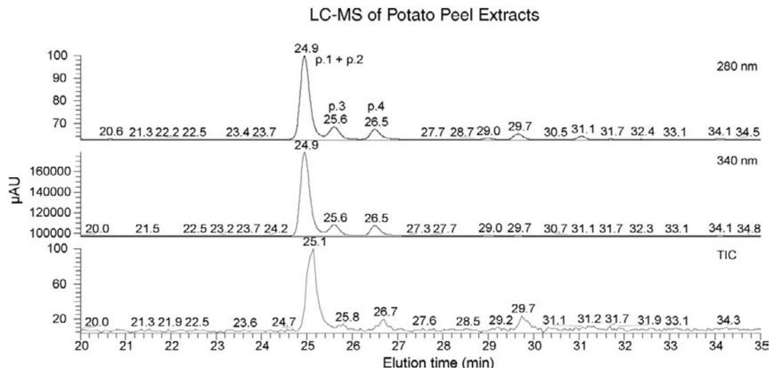
**Figure 6.7:** LC-MS chromatograms of an extract of Superior potato peel monitored at 280 nm, 340 nm, and TIC. Column: Inertsil ODS-3 (3  $\mu\text{m}$ , 4.0  $\times$  150 mm). Flow rate: 0.2 mL/min. Column temperature: 30°C. Mobile phase: acetonitrile: 0.5% formic acid (gradient mode).
