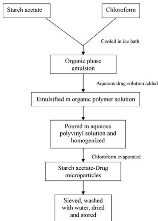
**Figure 16.2:** Preparation of starch acetate microparticles by water-in-oil-in-water double emulsion technique.
