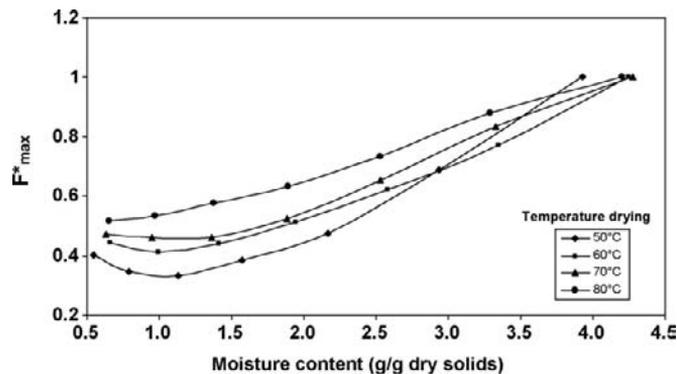
Figure 11.10: Changes in the  $F^*_{MAX}$  values with moisture content at different drying temperatures (reprinted with permission from J. Food Eng., 2007, 82, 577–584).
