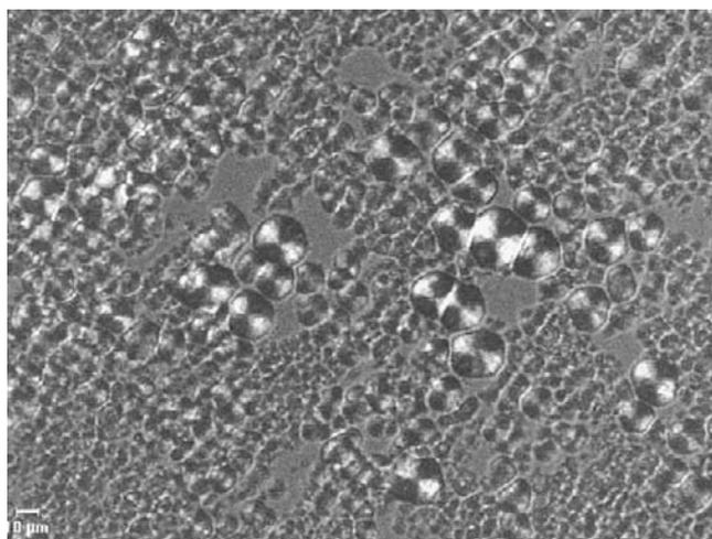
Figure 15.7: Morphology of aqueous potato starch dispersion (10%, w/w) heated to 180°C and quenched at 150°C/min to 10°C viewed between crossed polarizers. (Reprinted from: Ziegler et al., 2003, with permission from Elsevier).
