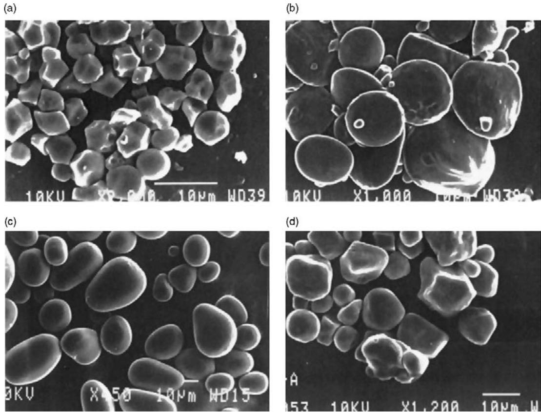
**Figure 10.1:** Scanning electron micrographs (SEM) of starches separated from different sources: (a) rice, (b) wheat, (c) potato, (d) maize (bar = 10  $\mu$ m) (source: Singh et al., 2003).
