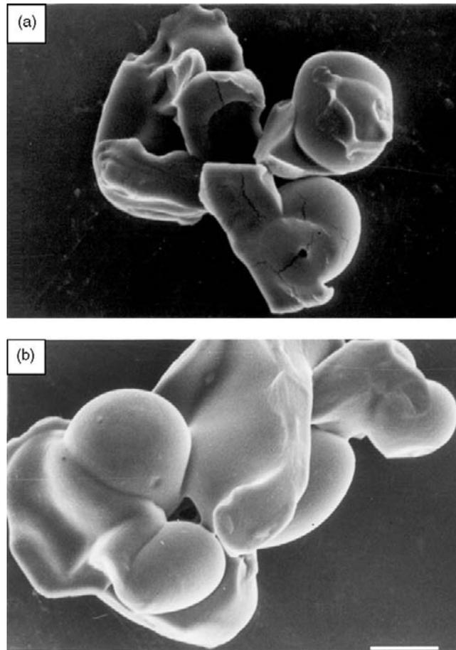
**Figure 10.5:** Scanning electron micrographs (a & b) showing granular indentation and fragmentation in granular cold water-soluble starches (source: Singh and Singh, 2003).
