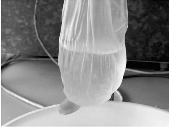
**Figure 15.3: Starch–clay nanocomposite bag made by film blowing technology. This bag has been stored filled with water and did not show any release nor failure after 3 weeks. (Reprinted from: Fischer, 2003, with permission from Elsevier).**
