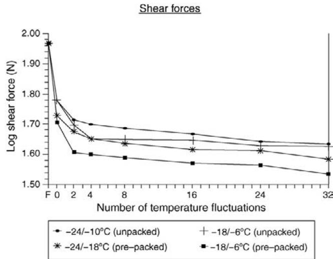
**Figure 7.8: Shear force (log scale) versus number of temperature fluctuations applied in the ranges  $-24$  to  $-18^{\circ}\text{C}$  and  $-18$  to  $-6^{\circ}\text{C}$  for unpackaged and pre-packaged frozen potato tissue.**
