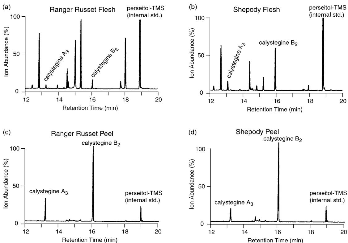
**Figure 6.4:** GC-MS total ion chromatograms of the hydrophilic alkaloid fraction extracted from freeze-dried potato flesh and peel.
