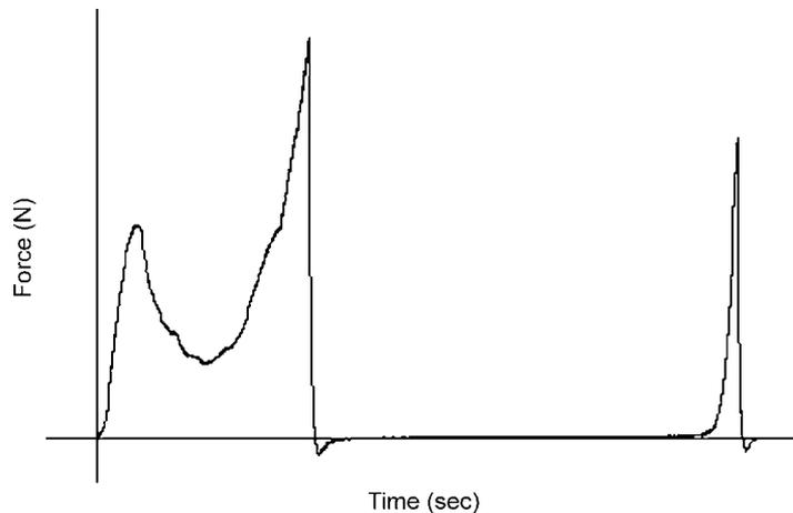
**Figure 9.4:** A typical texture profile analysis force-time curve for cooked potato. (Source: Singh et al., 2008).
