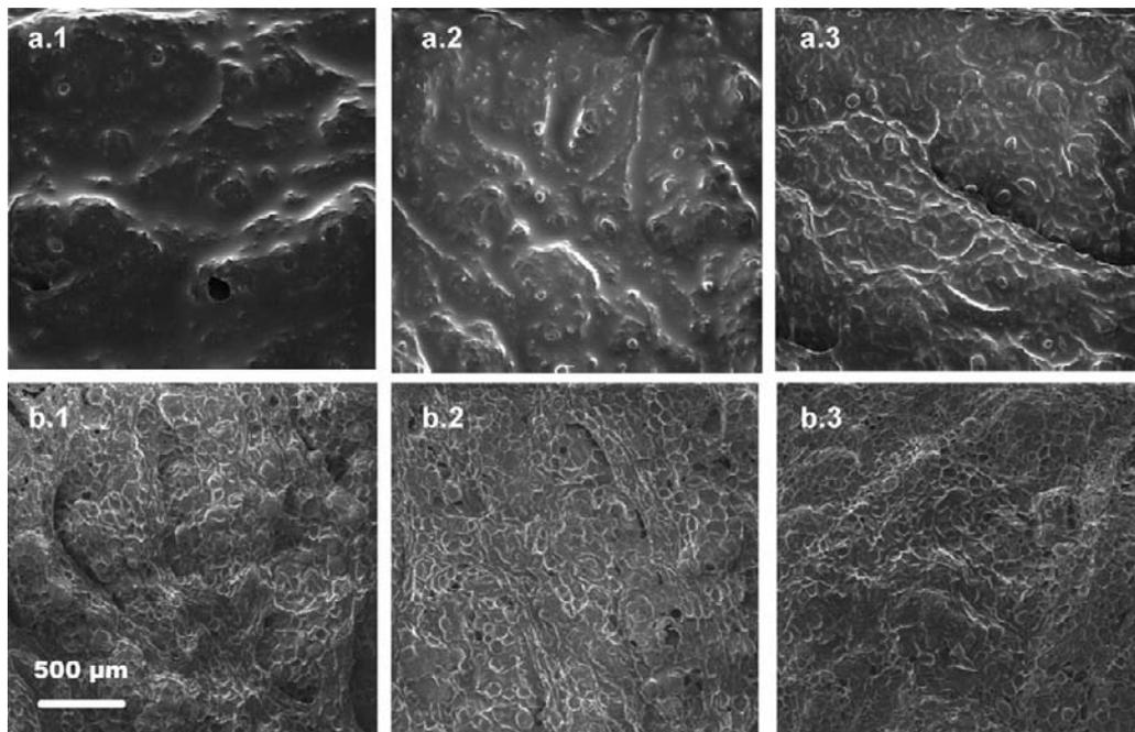
**Figure 11.5:** SEM images of the surface of control (a) and petroleum ether washed control for one second after frying (b) potato chips (moisture content  $\sim$  1.8%, total basis) fried at: (1) 120°C; (2) 150°C; (3) 180°C (reprinted with permission from *J. Food Eng.*, 2008, 87, 200–212).
