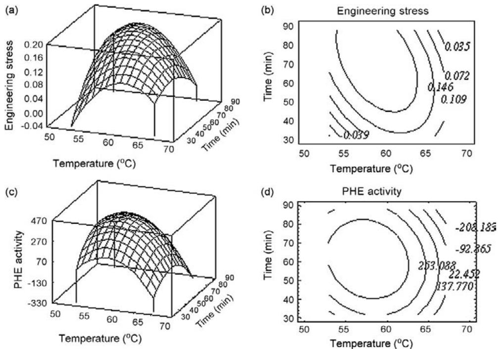
**Figure 7.15a-d: Engineering stress and PME activity response surfaces and contour plots as functions of blanching temperature and time. (a) Engineering stress response surface. (b) Engineering stress contour plot. (c) PME activity response surface. (d) PME activity contour plot.**
