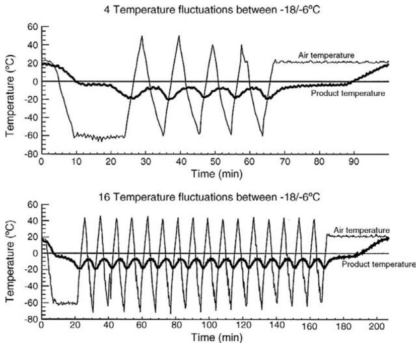
**Figure 7.7:** Thermal history of the product and of air temperature in unpackaged samples subjected to 4 and 16 fluctuations in the range  $-18$  to  $-6$  °C.
