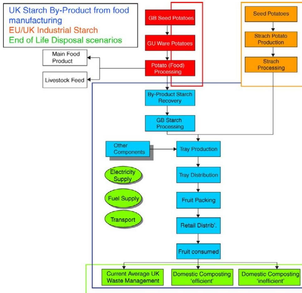
Figure 15.9: System boundaries of the Life Cycle Assessment of potato starch based packaging. (Reprinted from: Murphy et al., 2004, with permission from British Potato Council, UK).
