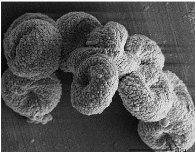
**Figure 15.8:** SEM image of spherulite aggregates of jet cooked high amylose starch dispersion slowly cooled without stirring. (Reprinted from: [Fanta et al., 2008](#), with permission from Elsevier).
