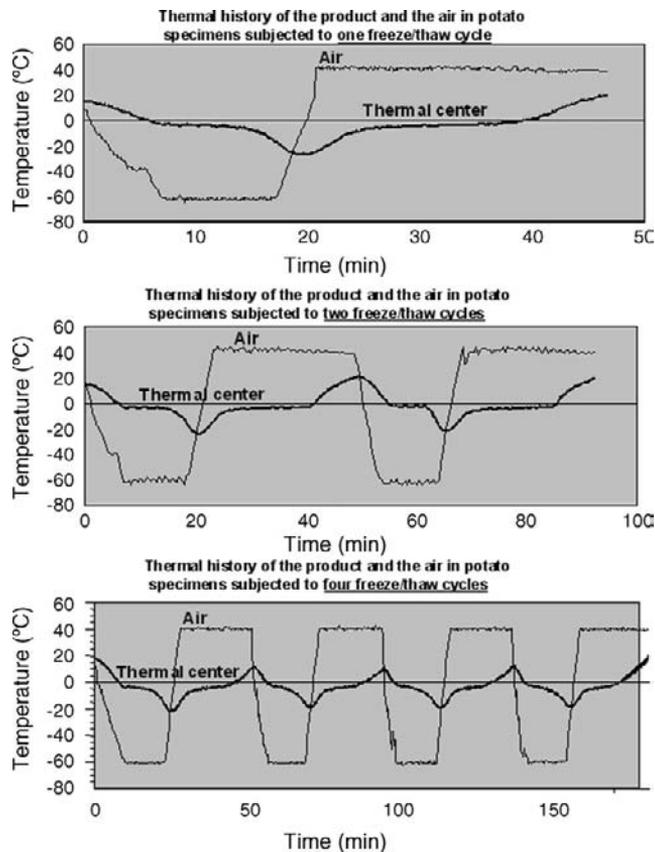
**Figure 7.5:** Thermal history of the product and of the air in potato specimens subjected to one, two, and four freeze/thaw cycles.
