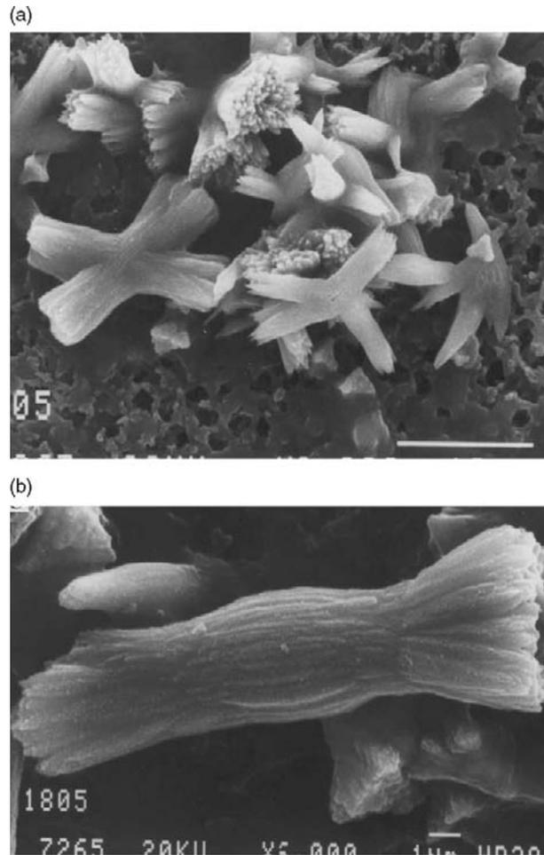
**Figure 10.8:** (a), (b) Rod-shaped microfibrils (showing longitudinal arrangement of crystalline structures) formed during long-term storage of hydroxypropylated gelatinized starch pastes (source: Kaur et al., 2004).
