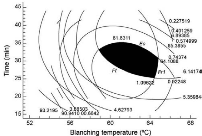
**Figure 7.11: Overlay of contour plots for apparent modulus of elasticity in compression ( $E_c$ ), maximum tension force ( $F_t$ ) and first-cycle relaxed force ( $F_{r1}$ ). The shaded area represents optimum conditions.**
