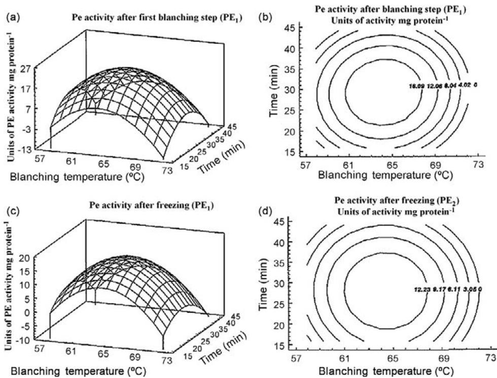
**Figure 7.13: PME activity response surfaces and contour plots as functions of blanching temperature and time.**
