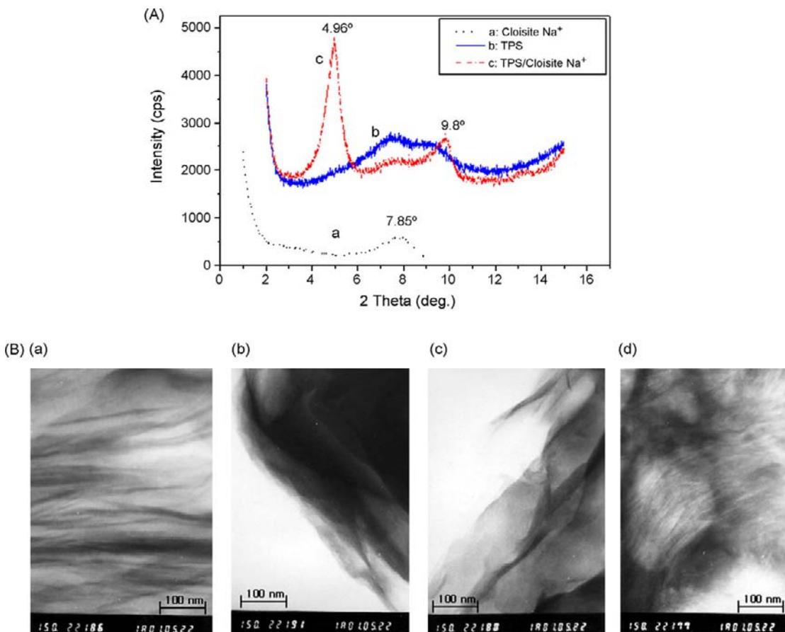
Figure 15.2: (A) XRD patterns of Cloisite Na<sup>+</sup> (a), Thermoplastic starch TPS (b), and the TPS/Cloisite Na<sup>+</sup> hybrid (c). (Source: Park et al., 2002). (B) TEM images of TPS/clay hybrids of different kinds of clay. (a) TPS95/Cloisite Na<sup>+</sup>, (b) TPS95/Cloisite 6A, (c) TPS95/Cloisite 10A, (d) TPS95/Cloisite 30B. (Reproduced with kind permission from: Park et al., 2002, ©Wiley-VCH Verlag GmbH & Co. KGaA).
