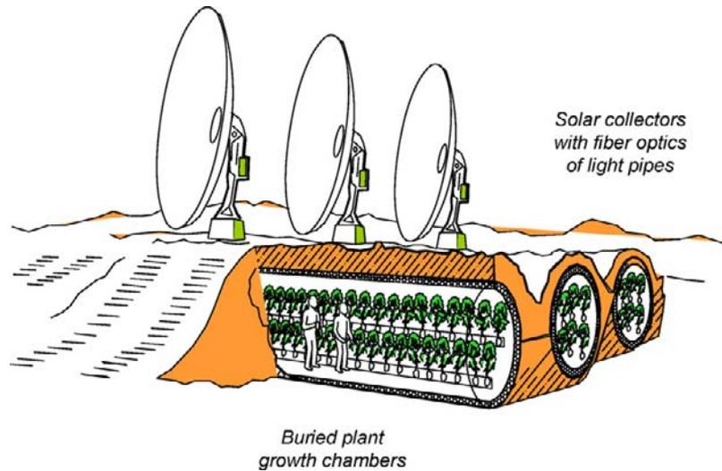
**Figure 17.22:** A concept of plant growth chamber covered with surface regolith for radiation shielding. Light could be collected with solar concentrators and piped into the plant chamber (source: [Sadler and Giacomelli, 2002](#)).
