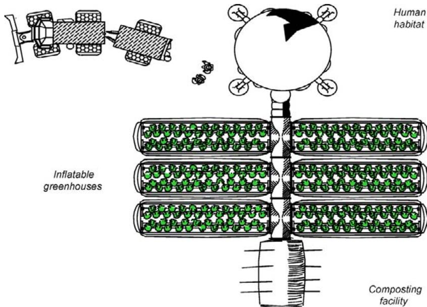
**Figure 17.21:** A concept for inflatable greenhouses (overhead view) that might be deployed on the surface of Mars (source: [Sadler and Giacomelli, 2002](#)). Inflatable structures are light weight and could be stowed in a small volume, but will require materials that are air tight, transparent, and tolerant of the UV radiation on the surface of Mars.
