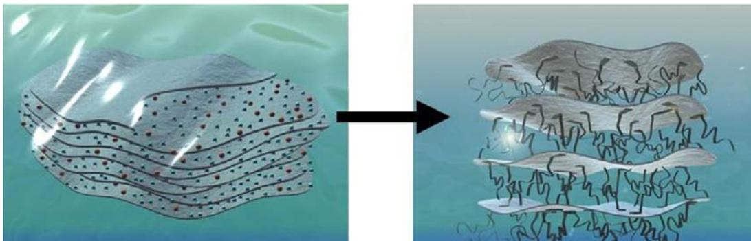
**Figure 15.6B:** Schematic picture of an ion-exchange reaction. The inorganic, relatively small (sodium) ions are exchanged against more voluminous organic onium cations. This ion-exchange reaction has two consequences: firstly, the gap between the single sheets is widened, enabling polymer chains to move in between them and secondly, the surface properties of each single sheet are changed from being hydrophilic to hydrophobic.
