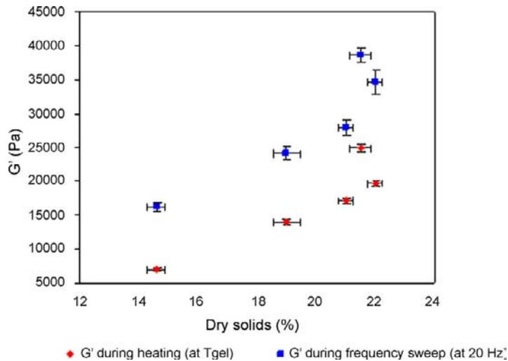
Figure 9.10: Effect of dry solids (%) on the storage modulus ( $G'$ ) of raw tuber flesh during temperature (heating) and frequency sweeps (Source: Singh et al., 2008).
