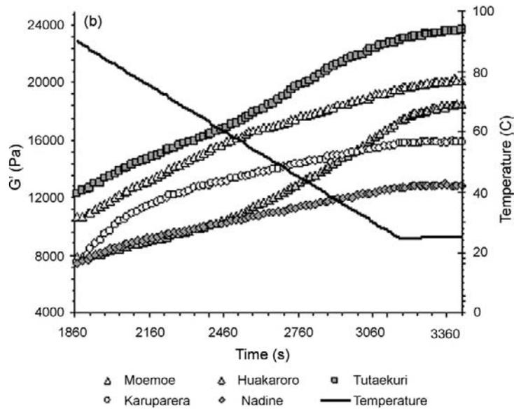
Figure 9.8b: Storage modulus ( $G'$ ) of raw tuber flesh during temperature sweeps (cooling). (Source: Singh et al., 2008).
