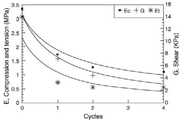
**Figure 7.6:** Models fitted for the effect of the number of freeze/thaw cycles on the apparent moduli of elasticity in the compression ( $E_c$ ) and tensile tests ( $E_t$ ), and on the modulus of rigidity ( $G_s$ ) in the shear test.
