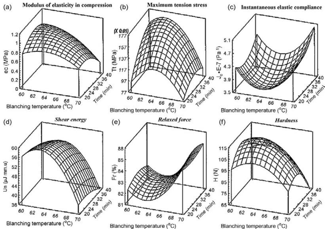
**Figure 7.14a–f:** Mechanical and textural property response surfaces as functions of blanching temperature and time. Steaming level: temperature 117 °C, time 2 min.
