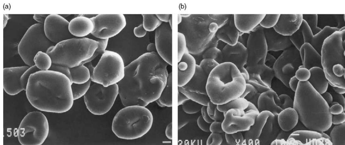
**Figure 10.6:** Effects of hydroxypropylation on the granule morphology of potato starches. (a) Potato starch granules after hydroxypropylation (at 10% propylene oxide concentration). (b) Effect of increased concentration of propylene oxide (15%) on the starch granule structure (source: Kaur et al., 2004).
