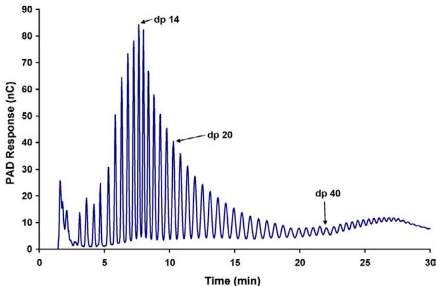
**Figure 8.1:** The profile of chain length and its distribution in potato starch by high-performance anion exchange chromatography (HPAEC).
