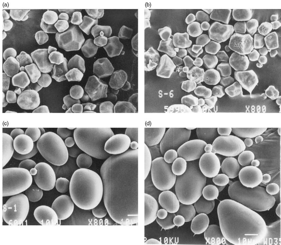
**Figure 10.9:** Effects of acetylation on the granule morphology of maize and potato starches. (a) Native maize starch granules. (b) Acetylated maize starch granules. (c) Native potato starch granules. (d) Acetylated potato starch granules (Singh et al., 2004a).
