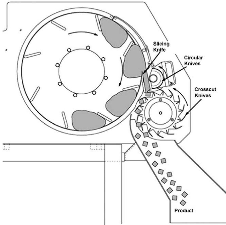
**Figure 7.2:** Diagram showing the operation schema of the DiversaCut 2110<sup>®</sup> Dicer by Urschel Laboratories, Inc. This equipment uniformly dices, strip cuts, and slices a wide variety of vegetables. (From Anonymous. How to cut fruits and vegetable products. Urschel laboratories incorporated. Valparaiso, Indiana, USA, with permission.)
