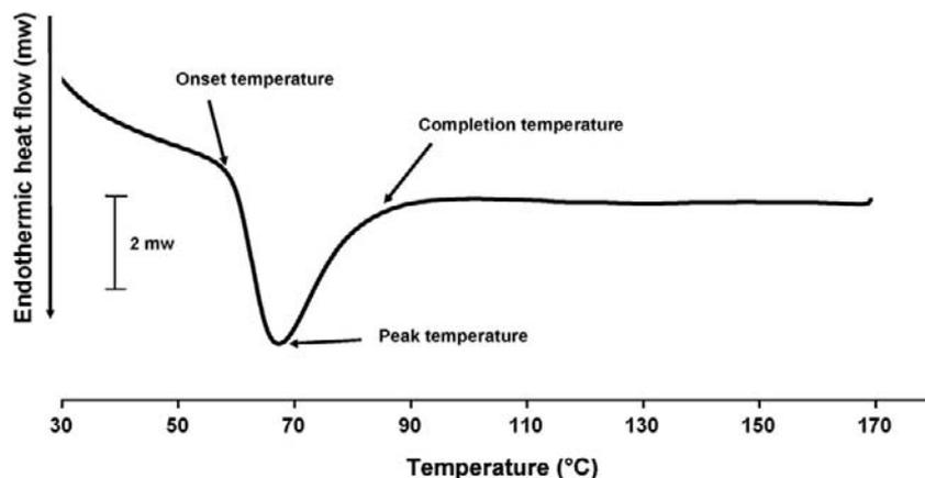
Figure 8.4: The gelatinization of native potato starch at 30% solid content by DSC.
