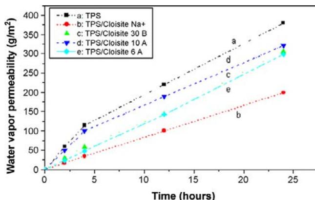
Figure 15.4: Water vapor permeability behavior of TPS/clay hybrids of different kinds of clays at 24°C. (Reproduced with permission from: Park et al., 2002, ©Wiley-VCH Verlag GmbH & Co. KGaA).
