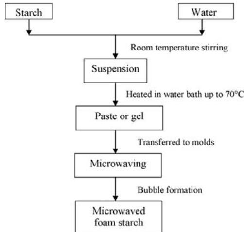
**Figure 16.1: Manufacturing of microwaved starch scaffolds (Torres et al., 2006).**
