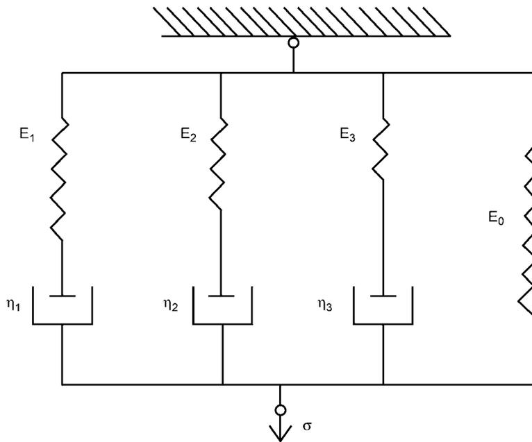
Figure 9.6: A seven element-Maxwell model representation for cooked potatoes.
