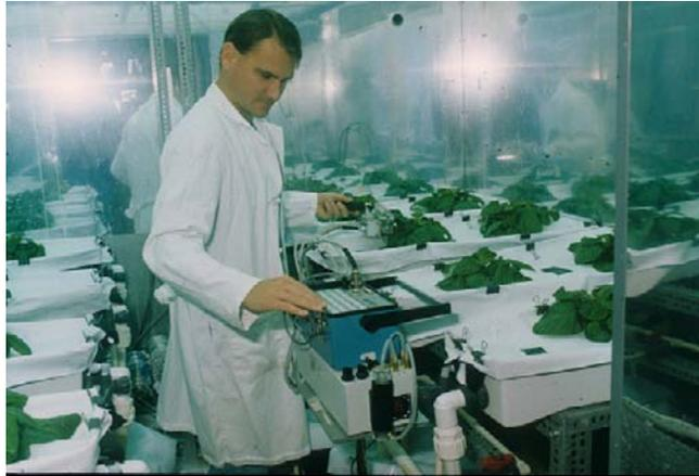
**Figure 17.11:** Neil Yorio at NASA's Kennedy Space Center taking leaf porometer measurements with potatoes to monitor stomatal conductance and transpiration rates. When measurements were taken at 400 ppm CO<sub>2</sub>, a mask was worn to removed exhaled breath from the chamber to avoid elevating the CO<sub>2</sub> concentration.
