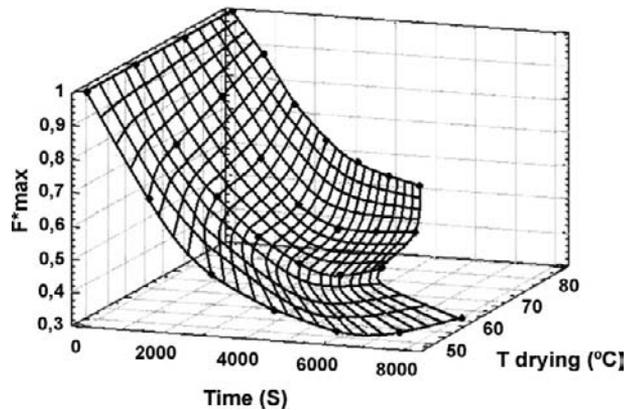
Figure 11.9: Changes in the  $F^*_{MAX}$  values of potato slices that air-drying at the different air temperatures tested (reprinted with permission from J. Food Eng., 2007, 82, 577–584).
