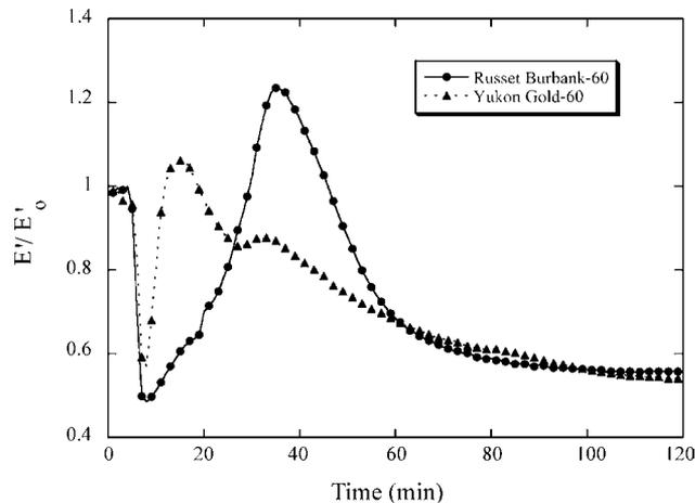
**Figure 9.7:** Profile of normalized storage modulus,  $E'/E'_0$ , of Russet Burbank potato disc as a function of heating time at 60°C;  $E'_0$  is the storage modulus of the raw sample = 1.87 MPa. (Source: Bu-Contreras, 2001).
