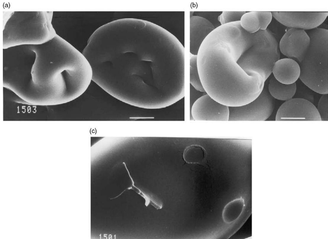
**Figure 10.7:** Effects of hydroxypropylation on the granule morphology of potato starches (at 10% propylene oxide concentration). (a), (b) Formation of deep groove in the central core region, folding of starch granules and formation of doughnut-like shape. (c) Formation of blister-like appearance and cracks on the starch granules (source: [Kaur et al., 2004](#)).
