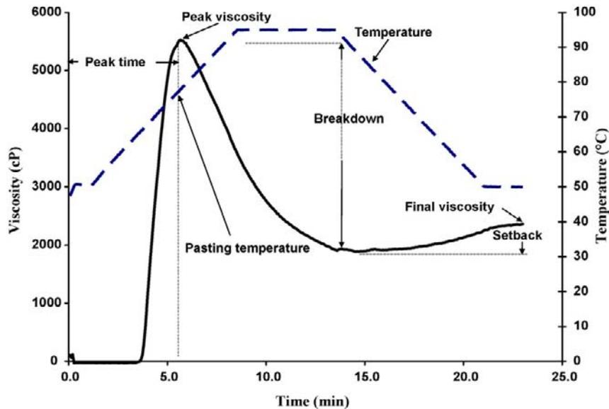
Figure 8.5: RVA pasting profile of potato starch.
