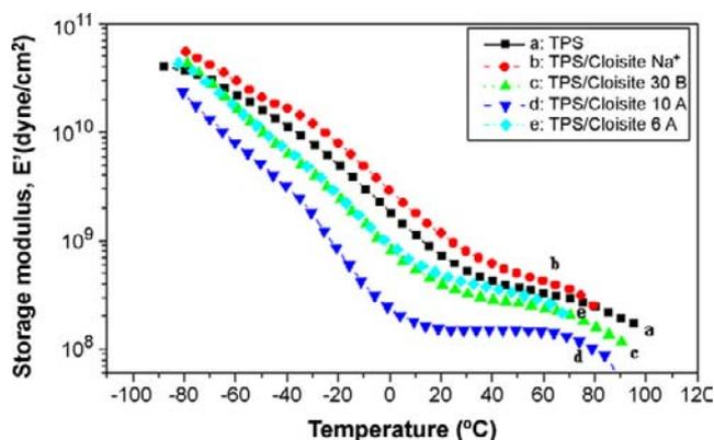
Figure 15.5: Typical storage modulus behavior of TPS/clay hybrids of different kinds of clays. (Reproduced with permission from: Park et al., 2002, ©Wiley-VCH Verlag GmbH & Co. KGaA).
