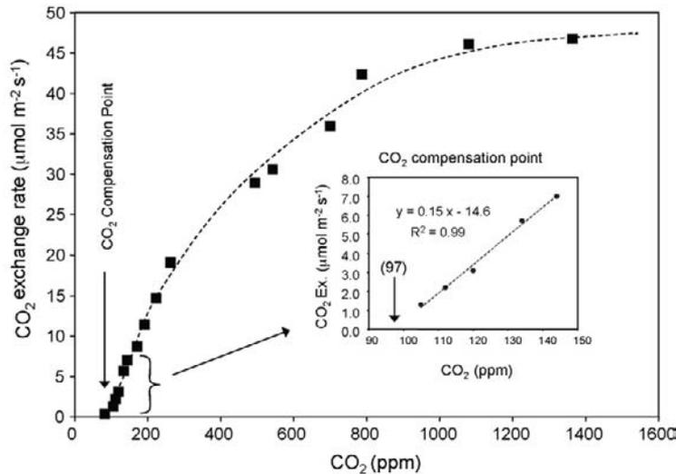
**Figure 17.15:** Carbon dioxide exchange rate (net photosynthetic rate) of a 20 m<sup>2</sup> potato stand at different CO<sub>2</sub> concentrations. The photosynthetic rates saturated above 1200 ppm while the CO<sub>2</sub> compensation point occurred at 97 ppm (source: Wheeler et al., 2008a).
