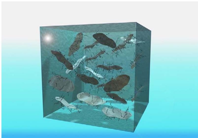
**Figure 15.1: Schematic picture of a polymer–clay nanocomposite material with completely exfoliated (molecular dispersed) clay sheets within the polymer matrix material. (Reprinted from: Fischer, 2003, with permission from Elsevier).**
