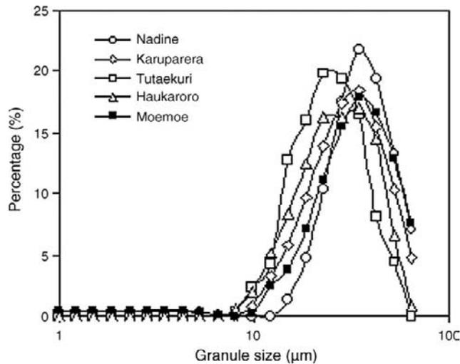
**Figure 10.2:** Particle size distribution of starches from some New Zealand potato cultivars (source: Singh et al., 2006).
