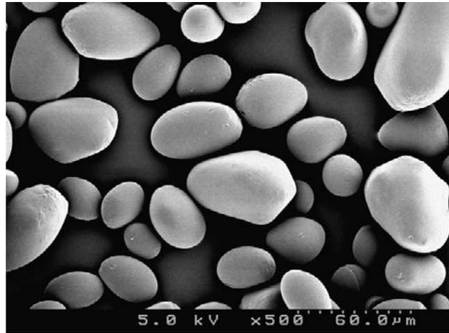
Figure 8.2: Scanning electron micrograph (SEM) of potato starch.
