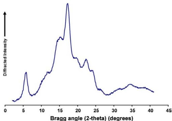
Figure 8.3: Wide angle X-ray diffraction profile of potato starch.
