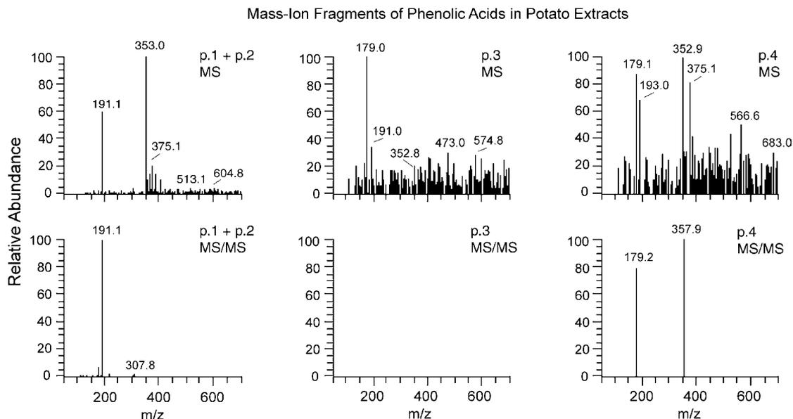
**Figure 6.9:** MS and MS/MS (negative ion mode) of peaks 1 and 2 (chlorogenic acid and its isomer), peak 3 (caffeic acid) and peak 4 (chlorogenic acid isomer) from isolated HPLC chromatograms of potato extracts.
