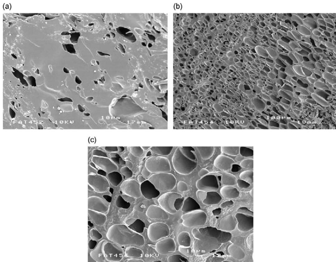
**Figure 15.6A:** Scanning electron micrographs (SEM) of fractured surfaces of (a) TPS-natural MMT nanocomposite containing 9.8 wt% clay, and (b) TPS-NH<sub>4</sub>MMT nanocomposite containing 10.7 wt% clay, (c) is the enlarged image for (b) showing spontaneously formed regular foam structures with 84% porosity in TPS-ammonium-treated clay.
