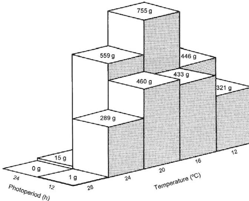
**Figure 17.9:** The effect of temperature on tuber yield from 56-day-old cv. Norland potato plants grown under 12 h or 24 h (continuous)  $400 \mu\text{mol m}^{-2} \text{s}^{-1}$  PAR. Peak yields under 12 h occurred at  $20^\circ\text{C}$ , while peak yields under 24 h occurred at  $16^\circ\text{C}$ . Few or no tubers were produced at  $28^\circ\text{C}$  (Wheeler et al., 1986a).
