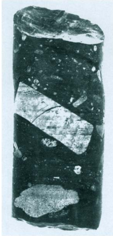
Fig. 4.26. A 5-cm-diameter core of Dwyka diamictite, Karoo basin, South Africa. Note the angularity of the clasts and the mud-supported fabric. This is a tillite formed during the Permo-Carboniferous glaciation of Gondwanaland.
