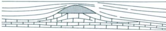
II Primary porosity dolomitization and fracturing in reefs ( Golden Lane, Mexico; Alberta, Devonian )
