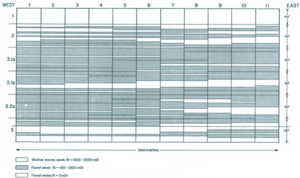
Fig. 6.12. (Upper) A conceptual cross-section through part of the Statfjord Formation (Triassic) petroleum reservoir in the northern North Sea showing the complex arrangement of reservoir sands, and nonreservoir shales. A blanket shallow marine sand at the top of the reservoir presents no problem, but note the problems of correlating and predicting sand continuity in the lower fluvial part of the section. In such reservoirs a probabilistic approach must be used. (Lower) Stochastic and other statistical methods are employed to produce a reservoir simulation model to compute the way in which the reservoir will produce petroleum (From Johnson and Stewart, 1985, by courtesy of the Geological Society of London).
