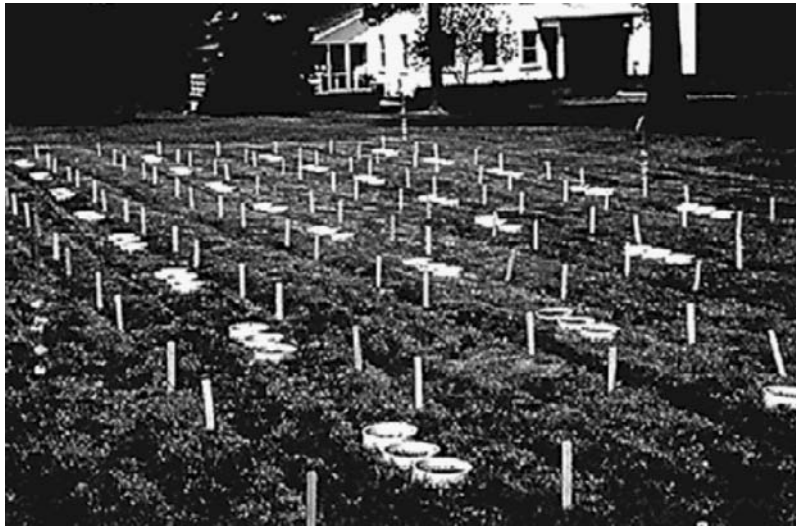
Figure 2. PVC cylinders in place for field test
