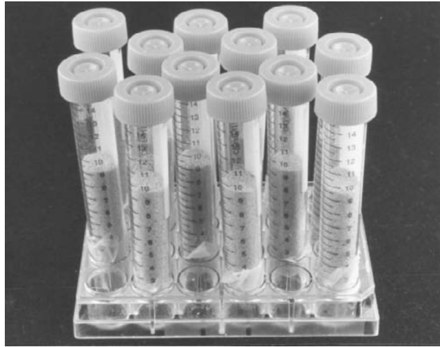
Figure 3. The bioassay unit used to test the efficacy and persistence of fungal conidial inocula applied to the soil surface
