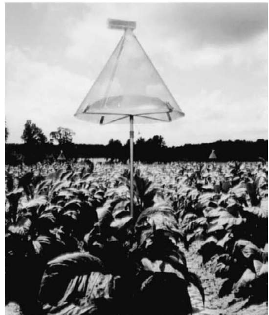
Figure 5. Photograph of plexiglass contamination station attached to a pheromone-baited wire-cone trap for autodissemination of nucleopolyhedroviruses
