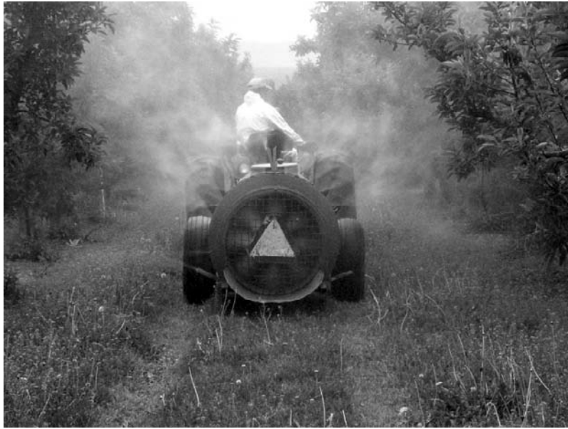
Figure 2. Tractor-pulled airblast sprayer configured for application of codling moth granulovirus. Photo by Steve Arthurs
