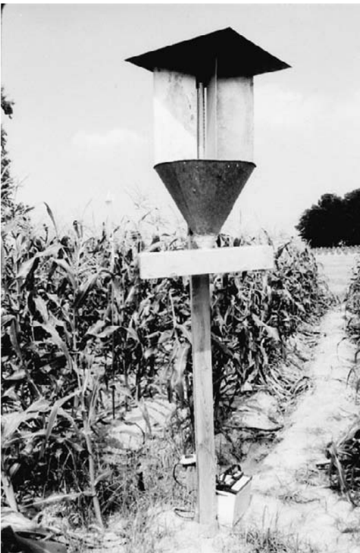
Figure 7. Photograph of aluminum contamination station attached to the bottom of a battery-powered blacklight trap for autodissemination of nucleopolyhedroviruses
