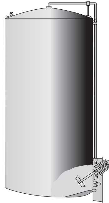
Figure 10.6 A tank with a propeller agitator. (Source: Dairy Processing Handbook , Tetra Pak.)
