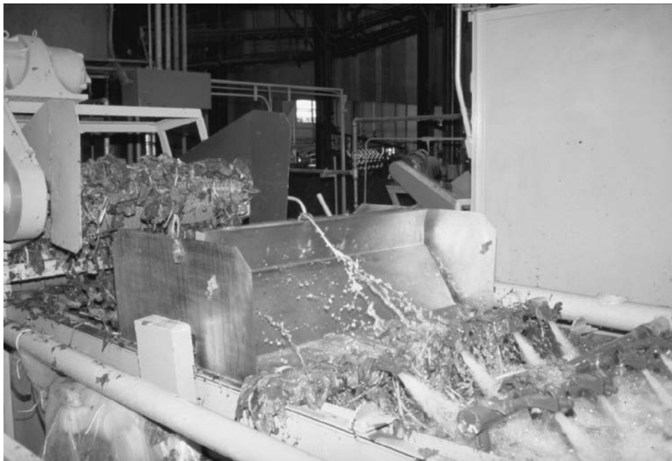
Figure 10.18 Water sprays are used in washing spinach. Leafy vegetables require a considerable amount of water to remove any insects and other debris attached to the leaves.
