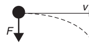
Figure 8.1b Constant vertical force F acting perpendicular to velocity v ; the particle trajectory (-----) will be parabolic.
