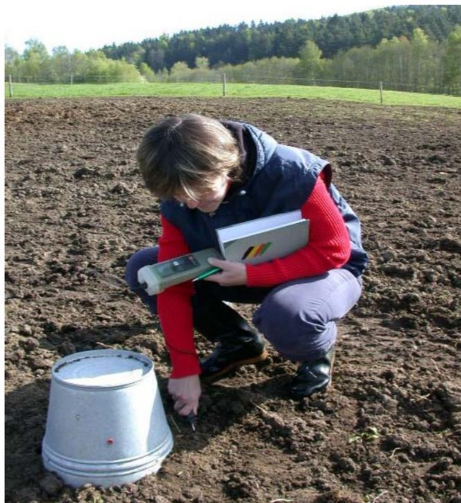
Figure 3. Flux and soil temperature measurements at the cattle overwintering area in 2004. The figure shows the chamber deployed to the severely impacted part of the area. The chamber covers ca 0.076 m<sup>2</sup> and its volume is ca 15 dm<sup>3</sup>. Notice the soil surface damaged by the animals.
