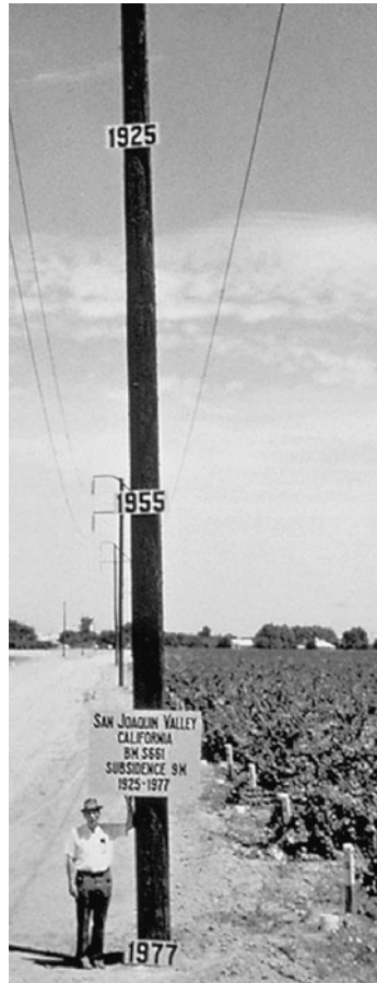
FIGURE 2.21 Approximate location of maximum subsidence in the United States identified by research efforts of Joseph Poland of the USGS (pictured). Signs on pole show approximate altitude of land surface in 1925, 1955, and 1977. The pole is near benchmark S661 in the San Joaquin Valley southwest of Mendota, CA (Galloway et al., 1999).
