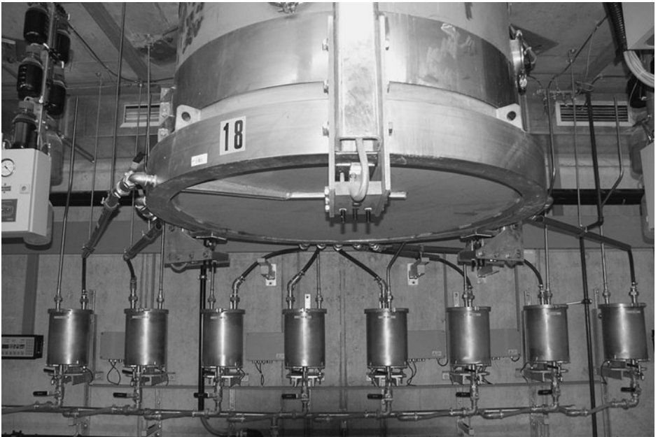
FIGURE 3.22 Below ground view of one of the lysimeters shown in Fig. 3.21. Various sensors and sampling equipment collect data for multidisciplinary studies, including water budget and groundwater recharge. (Photograph courtesy of Dr. Sascha Reth.)
