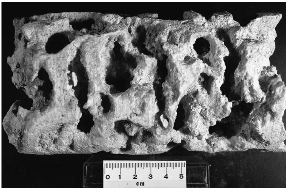
FIGURE 2.82 Large-diameter core from the Miami oolitic limestone (Biscayne aquifer), Miami, FL. Hydraulic conductivity \geq 1000 ft/d. (Photograph by George Sowers; printed with kind permission of Francis Sowers.)
