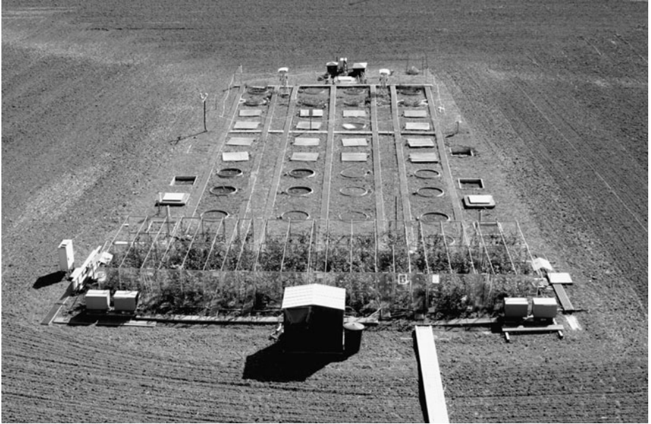
FIGURE 3.21 Array of lysimeters operated by Helmholtz Center Munich—German Research Center for Environmental Health (GmbH). (Photograph courtesy of Dr. Sascha Reth.)
