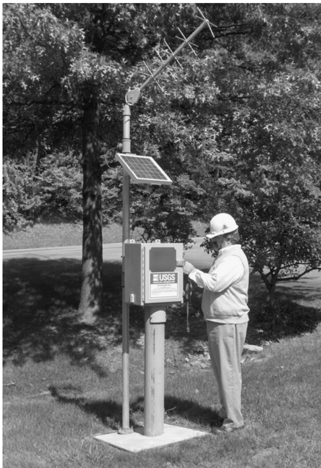
FIGURE 8.13 USGS monitoring well located at the headquarters of the National Ground Water Association in Columbus, OH. Water level data are recorded in real-time and transmitted via satellite to the USGS processing center. The data are available online 15 minutes after recording.
