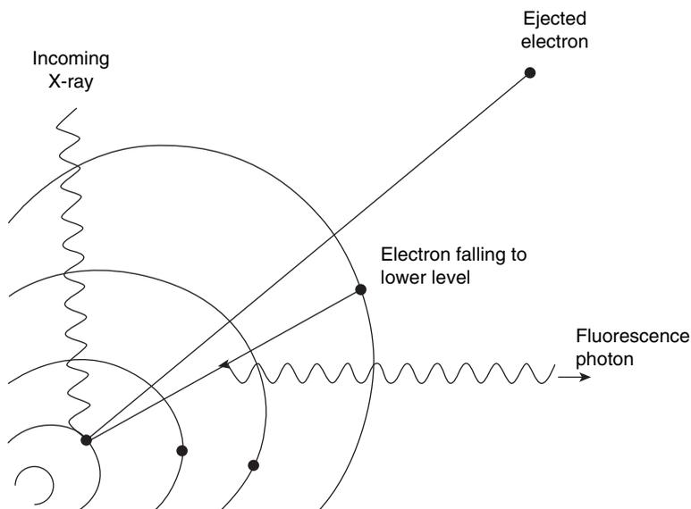
**Figure 8.3.** Diagram showing the source of X-ray fluorescence photons.
