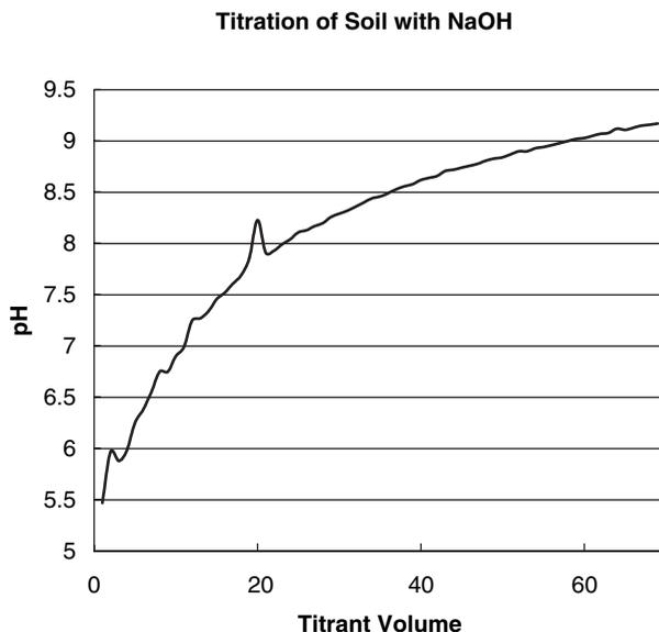
**Figure 6.5.** Titration of 50 g of soil suspended in 50 mL of distilled water with 0.1 M NaOH using a pH meter. Titrant was added slowly and continuously with stirring.
