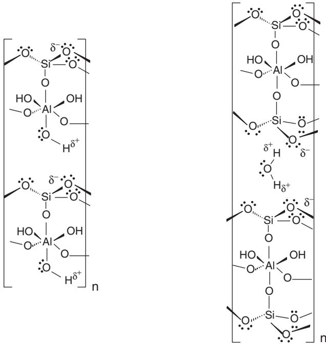
**Figure 2.2.** The left structure represents kaolinite, a 1:1; and the right, a 2:1 clay mineral. These representations are intended to show surface groups, surface pairs of electrons, unsatisfied bonds, and associations between clay particles. Note that clay structures are three-dimensional and these representations are not intended to accurately represent either the three-dimensional nature or the actual bond lengths; also, the brackets are not intended to represent crystal unit cells.
