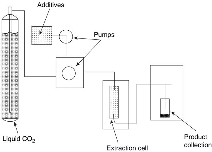
**Figure 7.6.** Setup for supercritical extraction of soil.
