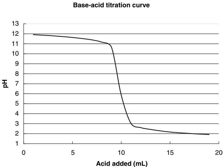
**Figure 6.1.** Curve obtained titrating a standard base with a standard acid.
