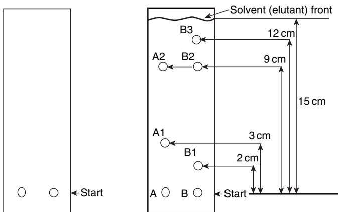
**Figure 9.8.** Thin layer at start (left) and after development (right). Right chromatogram shows the distance that the elutant and spots moved during the development of the chromatogram.
