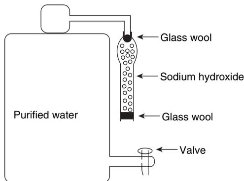
**Figure 7.1.** Purified water container protected from carbon dioxide by a drying tube containing sodium hydroxide (*Caution:* adsorption of water by  $\text{NaOH}$  produces caustic solution).
