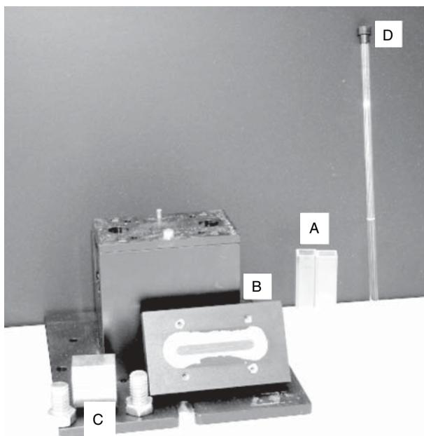
**Figure 8.7.** Sample holders for various spectrophotometric measurements: (A) UV-Vis cells; (B) infrared attenuated total reflection (ATR) plate and stand—plate is attached to stand behind it when in use; (C) simple KBr pellet maker using the two bolts and the center dye; (D) a sample tube for NMR spectroscopy.
