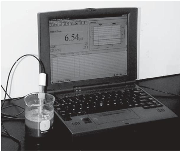
**Figure 5.6.** A pH electrode in a soil suspension. The electrode is connected to a computer that shows the readout.
