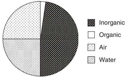
**Figure 1.8.** Idealized general composition of a soil sample.
