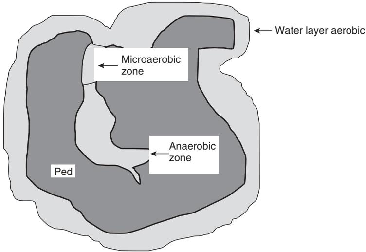
**Figure 4.5.** Aerobic, microaerobic, and anaerobic zones in a soil ped.
