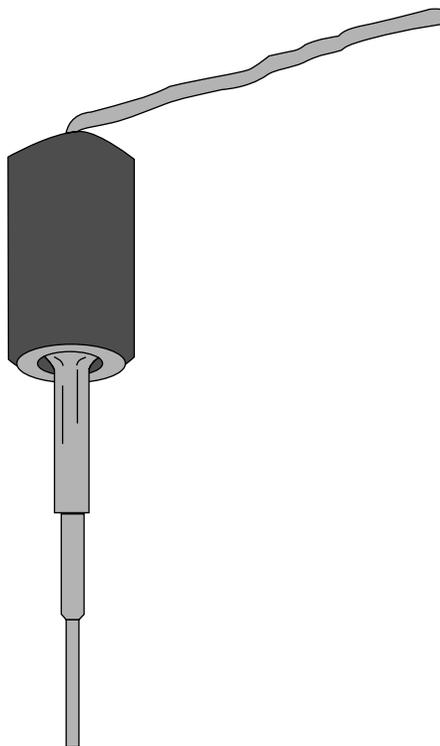
**Figure 7.4.** Ultrasonic “horn” for disruption and extraction of soil samples.
