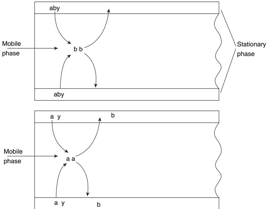
**Figure 9.1.** Partitioning of the components of a mixture in a chromatographic column.
