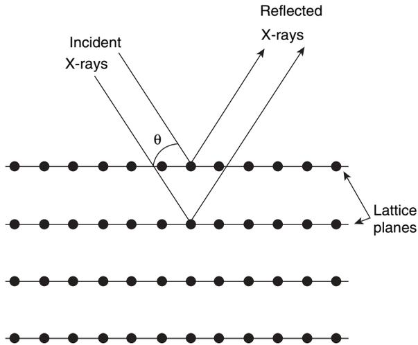
**Figure 8.2.** The diffraction of X rays from crystal planes.
