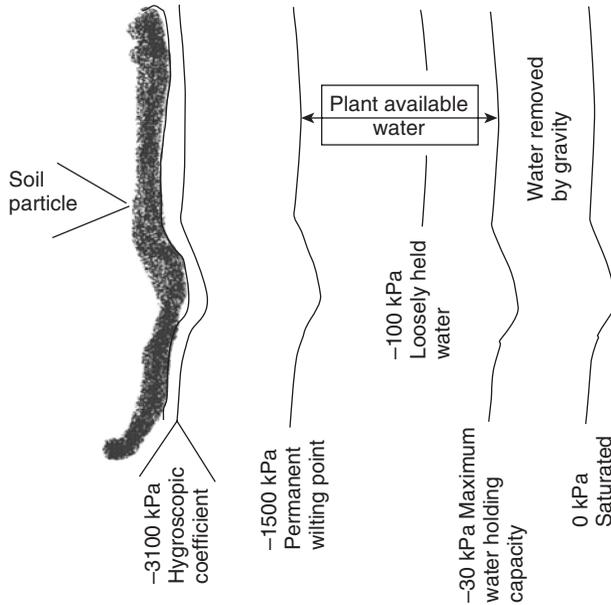
**Figure 4.2.** Potential of "layers" of water surrounding a soil particle.
