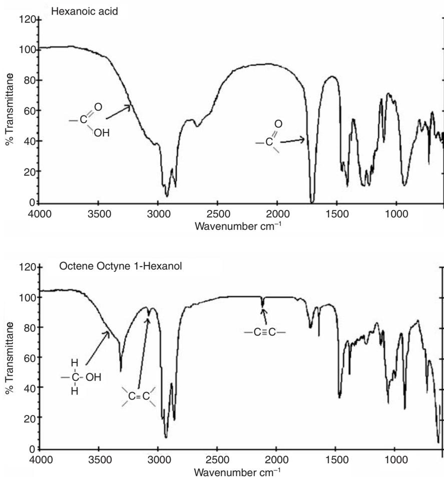
**Figure 8.11.** Infrared spectra showing common absorption. Both the OH of acids and alcohols are hydrogen-bonded, leading to broadening of the absorption. Note that the OH absorption of hexanol is unusually sharp for a hydrogen-bonded alcohol.
