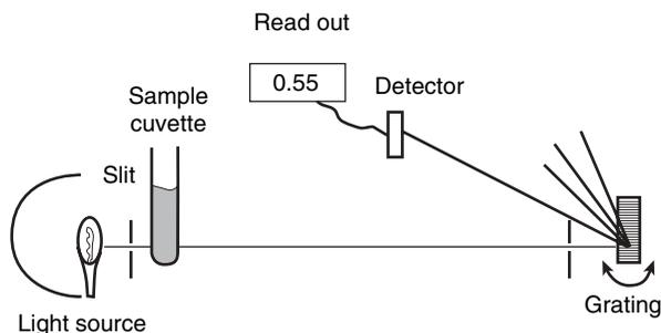
**Figure 8.8.** Diagram of the light path in a spectrophotometer.
