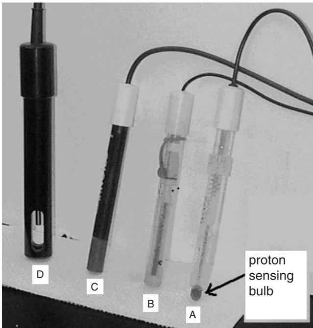
**Figure 5.5.** A combination pH electrode is shown (A). The dark-colored tip is the pH sensing glass electrode. The reference electrode is not visible. A reference electrode (B) for ISE measurement along with a nitrate-selective electrode (C) are also shown. Electrode D is used for measuring salt content in aqueous solutions.
