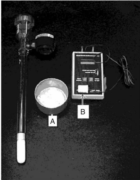
**Figure 4.9.** Shown from left to right are a tensiometer, soil drying can (A) and porous block (B) and meter for determination of soil water.
