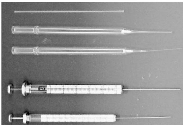
**Figure 9.3.** Sample application tools from top to bottom, glass capillary, Pasteur pipette with tip drawn out, syringe for HPLC, and syringe for GC.
