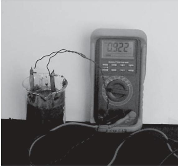
**Figure 5.1.** Zinc and copper strips inserted into wet soil and producing a voltage as shown on the voltmeter.
