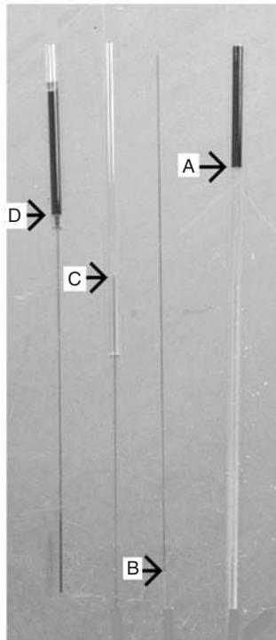
**Figure 4.3.** A wide-diameter capillary tube (A) draws colored a shorter distance than does a narrow-diameter capillary (B). Colored water cannot move from the narrow-diameter capillary to the wide-diameter capillary (C). Colored water can move from a larger diameter capillary to a smaller capillary (D).
