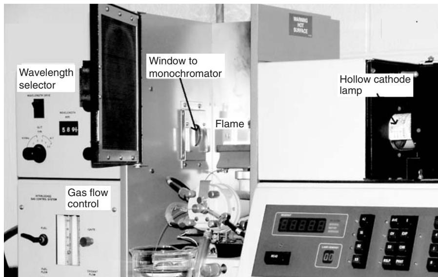
**Figure 8.4.** An atomic absorption spectrophotometer capable of functioning in either the EM or AA mode.
