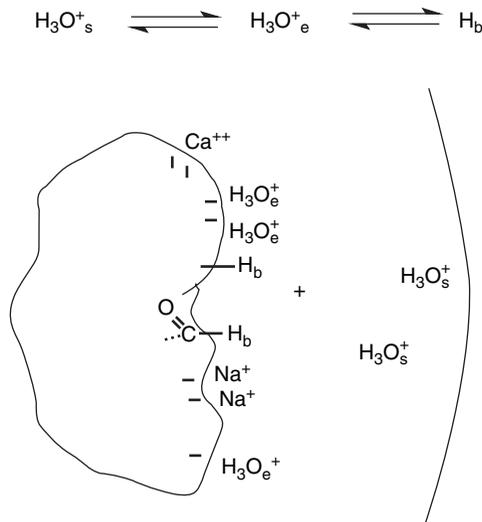
**Figure 6.4.** An equation showing the equilibrium between bonded protons ( $\text{H}_b$ ), exchangeable protons ( $\text{H}_3\text{O}^+_e$ ), and soluble protons ( $\text{H}_3\text{O}^+_s$ ) is given above and illustrated below.
