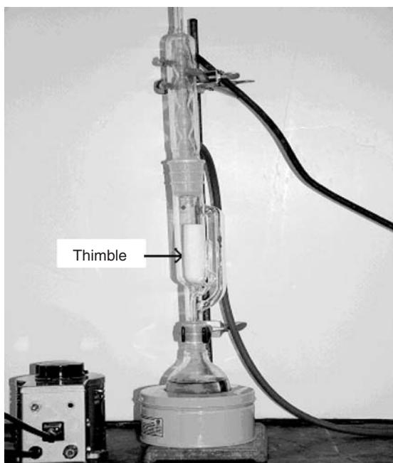
**Figure 7.2.** Soxhlet setup for extraction of solid samples.
