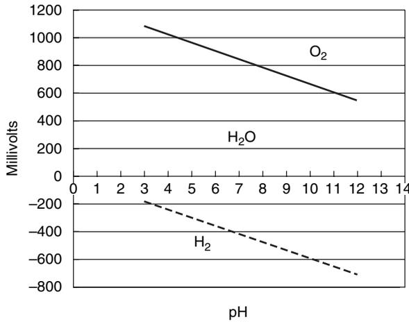
**Figure 5.3.** Electrode potentials for the oxidation of oxygen and the reduction of hydrogen at gaseous pressure of 1 atm and pH levels common in soil.
