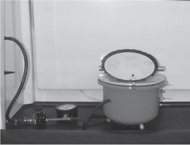
**Figure 4.10.** Pressure apparatus for measuring the amount of water held in soil at different pressure; pressure gauge is to the left, and a pressure plate is on top of the vessel.
