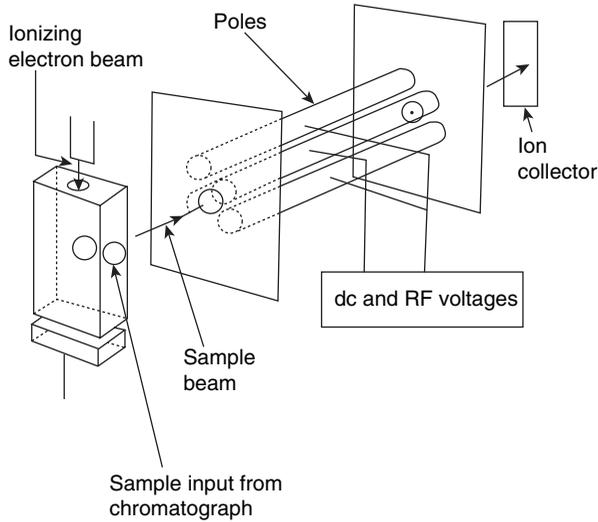
**Figure 9.5.** Diagram of quadrupole MS used as detector for gas chromatography.
