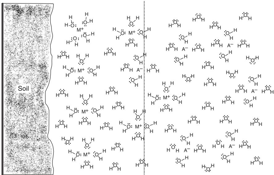
**Figure 4.8.** A soil particle with a diffuse layer of hydrated ions around it. The dashed line represents the boundary of the layer of tightly held cations. This diagram is not meant to be an exact representation of the diffuse double layer around a soil particle.
