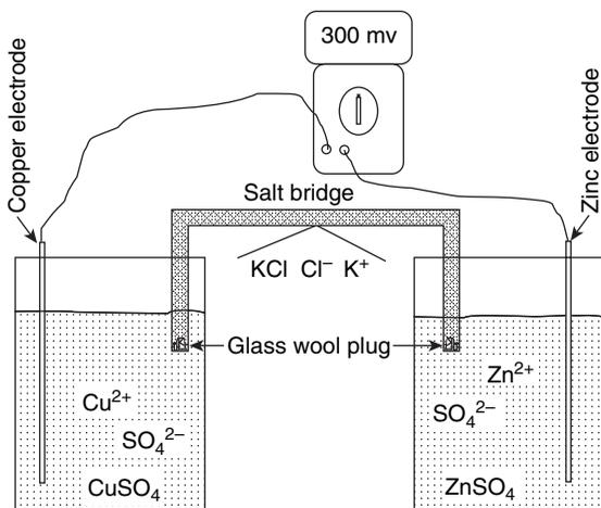
**Figure 5.2.** A typical electrochemical cell.
