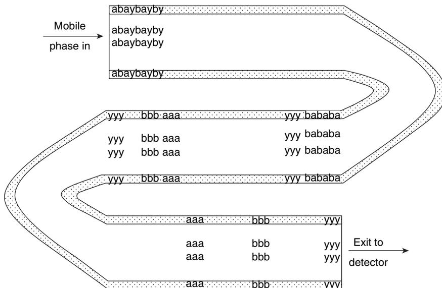
**Figure 9.2.** Separation of a complex mixture by chromatography. The top segment shows the column just after application of mixture. As the sample progresses through the column, separation of mixture occurs as a result of the chromatography. The first component exits the column and is detected, followed by the other two components.
