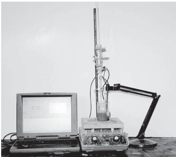
**Figure 6.2.** Setup for titrating and recording pH change using a pH meter card in a laptop computer.
