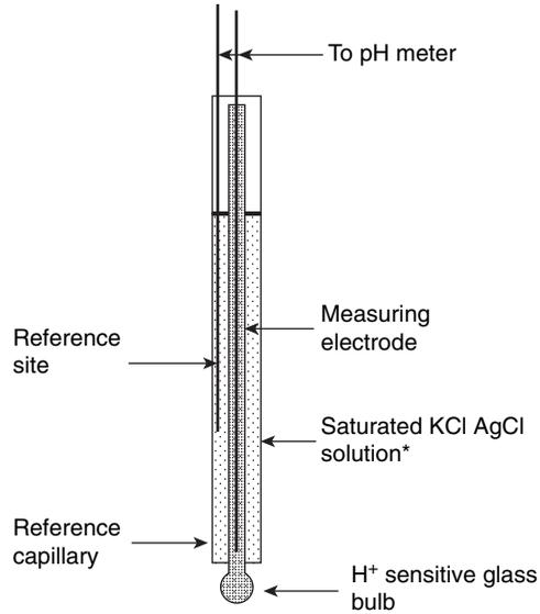
**Figure 5.4.** Typical setup for a combination pH electrode. Note that the saturated KCl/AgCl solution can be different depending on the electrode manufacturer.
