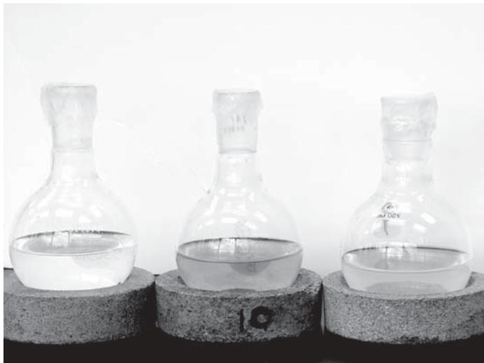
**Figure 7.3.** Solutions obtained by Soxhlet and magnetic stirring of soil with either water or hexane.
