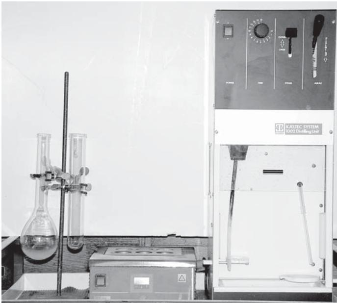
**Figure 6.6.** Setup for performing kjeldahl analysis of soil. On the left are two different types of kjeldahl flask; to the right of the flask is a heating block used to heat the text-tube-shaped flask during digestion and on the right, a steam distillation unit.
