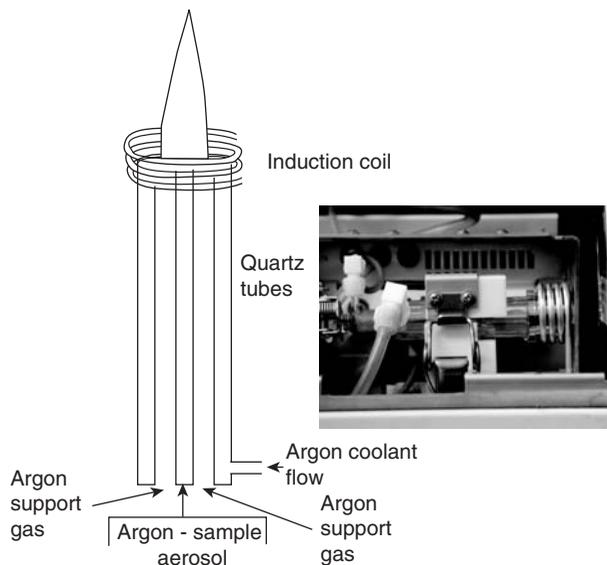
**Figure 8.5.** Left is a diagram and on the right is a photograph of an ICP torch.
