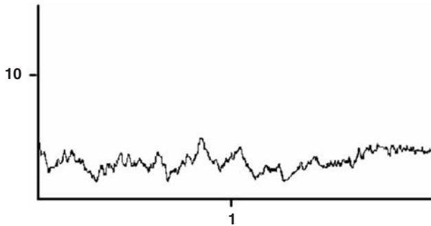
**Figure 8.1.** Baseline noise from a gas chromatograph.
