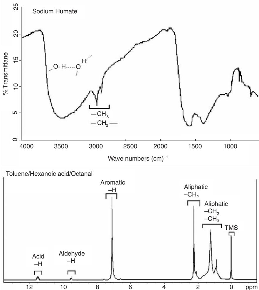
**Figure 8.12.** Infrared spectra of a KBr pellet of 3% sodium humate (Aldrich) and an NMR spectrum of a mixture of toluene, hexanoic acid, and octanal. The functionalities responsible for the absorptions are labeled.
