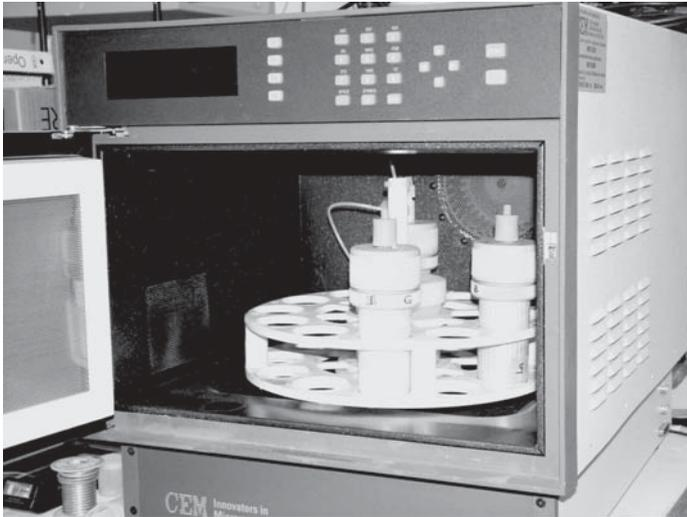
**Figure 7.5.** A microwave-assisted instrument showing extraction vessels and attachment for sensors (courtesy of Dr. Corso and Dr. Conklin, University of Cincinnati).
