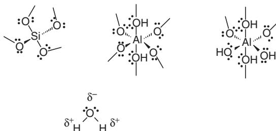
**Figure 2.1.** A silicon tetrahedron (left), an aluminum octahedron as a central layer in a 2:1 clay and an aluminum octahedron as a surface layer in a 1:1 clay (right). Both the oxygen and OH groups are bonded to other silicon and aluminum atoms in the clay (bonds are not intended to be shown at the correct angles). Below is a water molecule showing partially positive hydrogens and partially negative oxygens. Also shown are the two lone pairs of electrons on all the oxygens.
