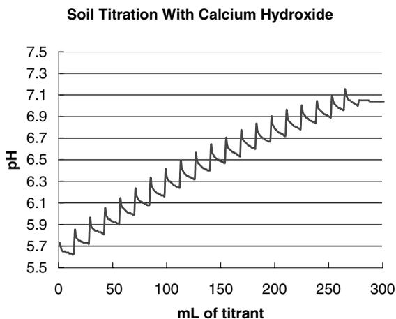
**Figure 6.3.** Stepwise titration of acidic soil with calcium hydroxide.
