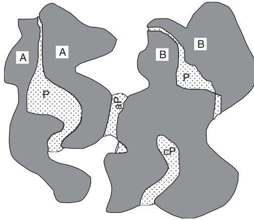
**Figure 4.4.** Two pedes (*AA* and *BB*) each have a pore that does not drain because the mouths are too small. Ped *BB* has a pore closed at one end (i.e., *cP*). Between the pedes is an apparent pore (*aP*) formed by the close proximity of the pedes.
