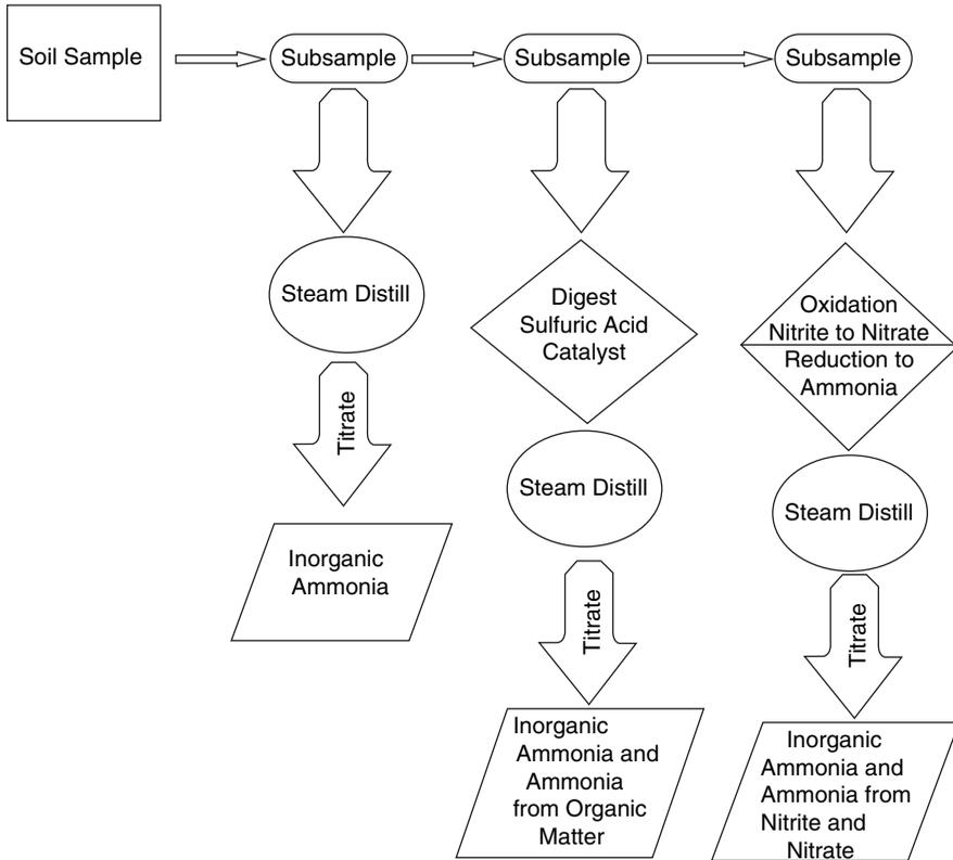
**Figure 6.7.** Flow diagram for determination of ammonia, organic nitrogen, nitrite, and nitrate using kjeldahl apparatus [6].
