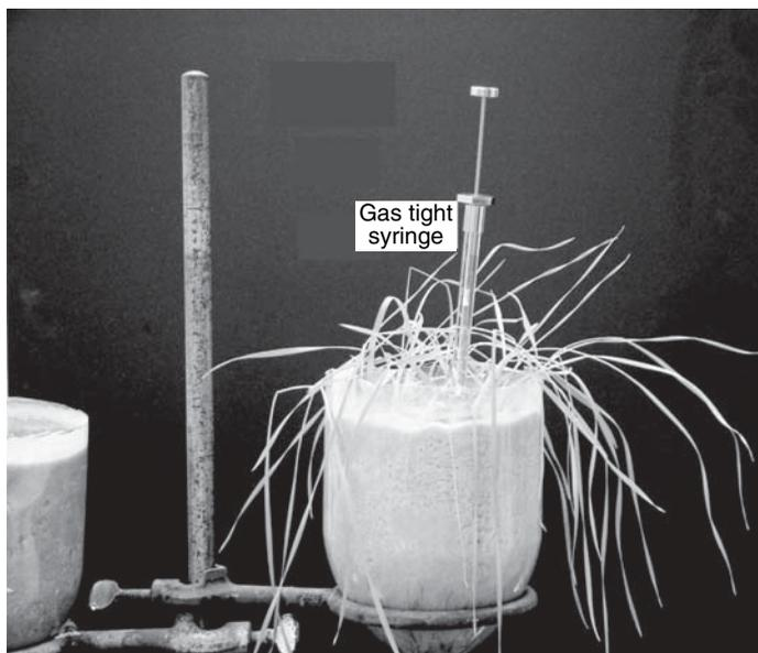
**Figure 9.7.** Gastight syringe used to sample soil air; the same chromatograph is shown in Figure 9.6.
