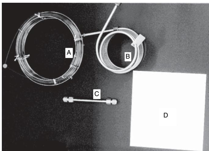
**Figure 9.4.** Columns used in chromatography and a thin-layer sheet. Columns *A* and *B* are a capillary column and a packed column, respectively. Column *C* is for HPLC. Column *D* is a thin-layer sheet with plastic backing such that it can be cut into smaller pieces as needed.
