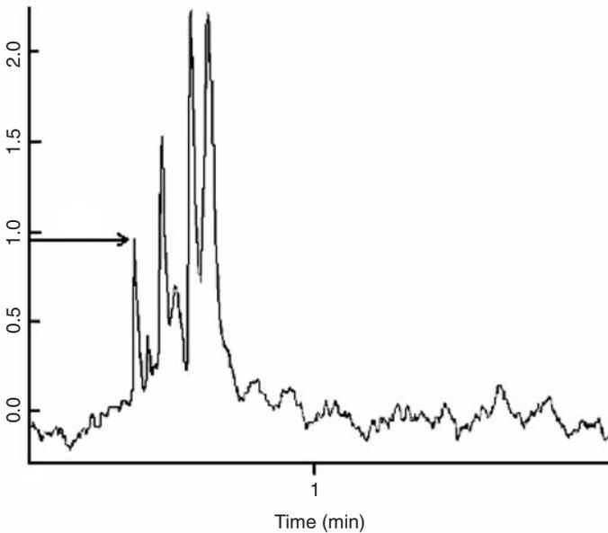
**Figure 9.6.** Gas chromatograph of soil air taken in Figure 9.7.  $R_t$  is the time it takes the first peak to come out.  $R_t$  values can be found for all peaks if needed.
