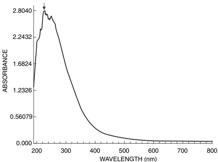
**Figure 8.6.** UV-Vis spectrum of simple deionized water extract of soil. Absorption maximum is indicated by an arrow. Note that the absorbance is above 1, and therefore the solution should be diluted before attempting to interpret the spectrum.
