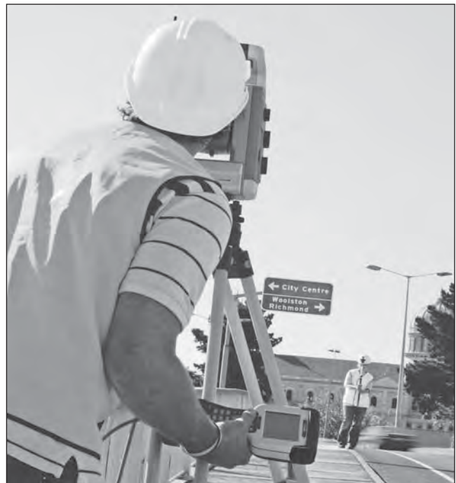
FIGURE 14.2 Total station, data collector, and prism. (Photo courtesy of Trimble © 2008)
