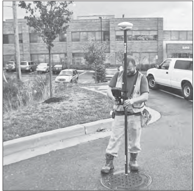
FIGURE 14.6 RTK rover and data collector. (Photo courtesy of Sam Dougherty and Steve Hall of Dewberry and Trimble © 2008)
