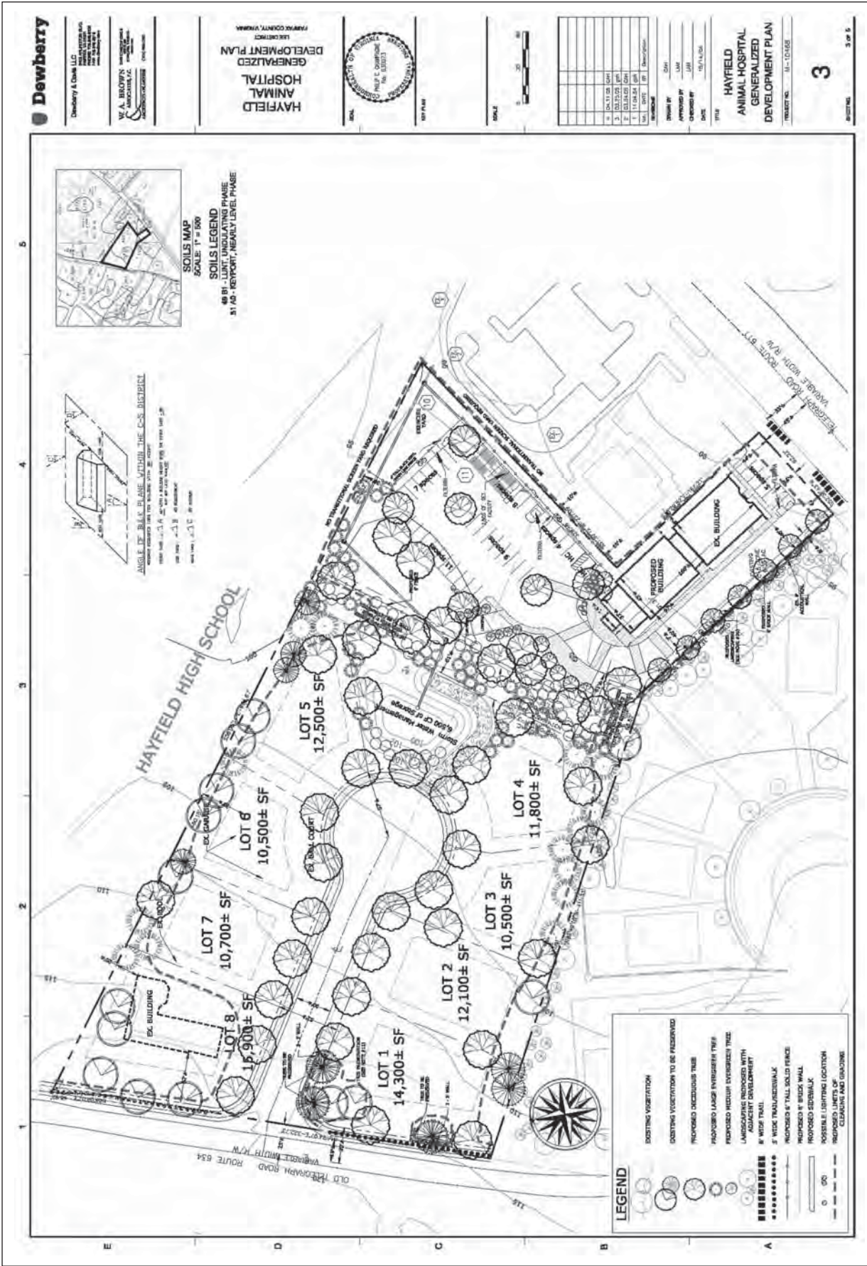
FIGURE 19.1 Example of a preliminary site plan.
