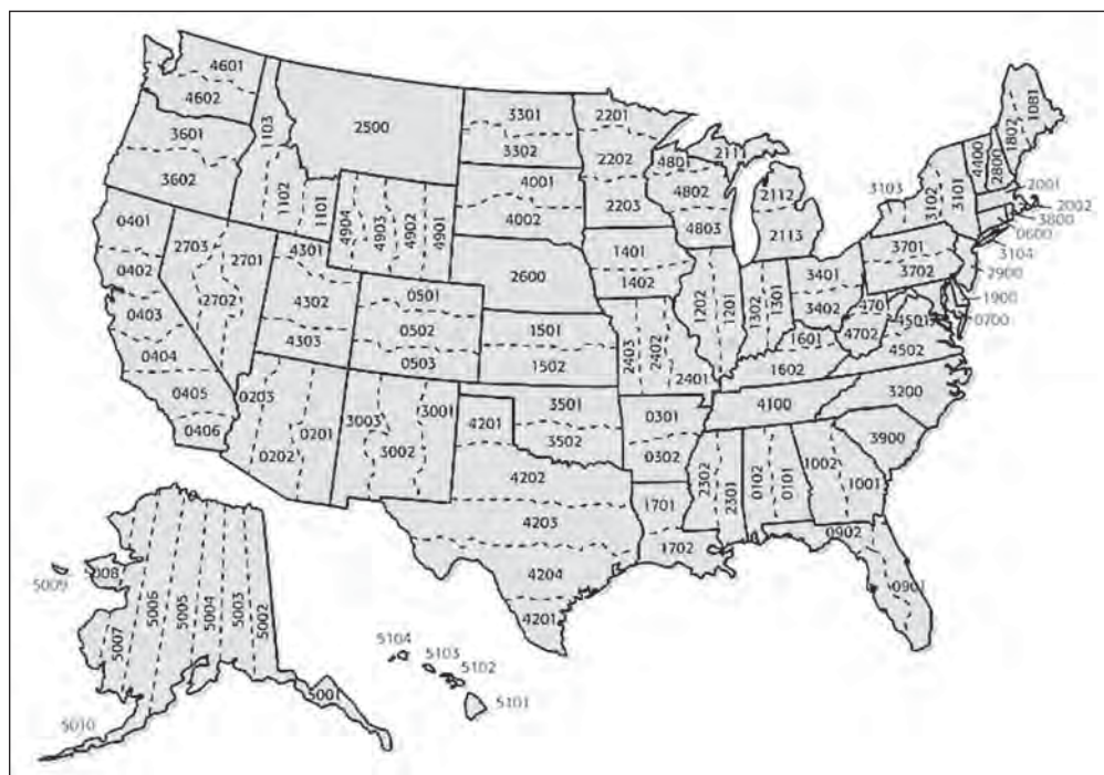
FIGURE A.9 With few exceptions (e.g., Montana and Nebraska), most states have adopted a State Plane Coordinate System to keep scale factors between 0.99990 and 1.00010 so that scaling errors will be 1:10,000 or less. Generally speaking, states longer in the north-south direction utilize one or more transverse Mercator zones, whereas states longer in the east-west direction utilize one or more Lambert conformal conic zones. Zone boundaries normally curve to coincide with county boundaries in order to keep entire counties within a single zone.
