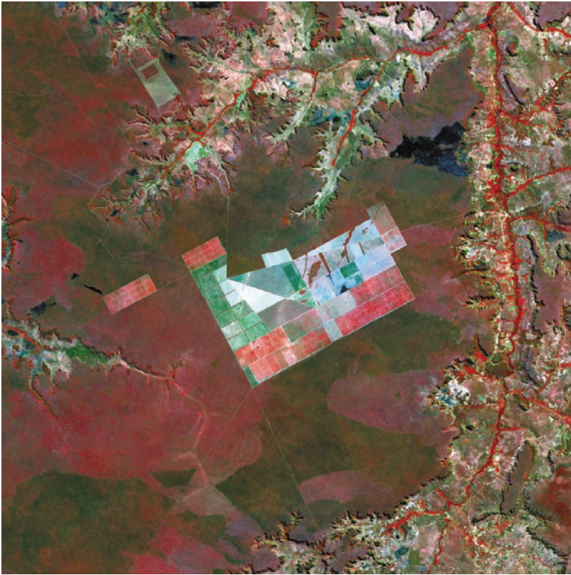
Fig. 4.10. Landsat TM 5 image referred to Rondonia, Brazilian Amazonian rainforest. This is a color composite of bands 4, 5, and 3. Primary forests and converted land uses are evident
