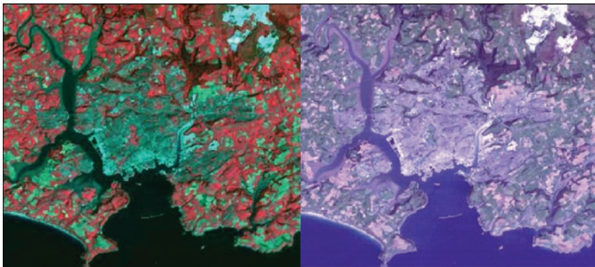
Fig. 4.6. Landsat Thematic Mapper ( TM ) images. Near-IR left ) shows a very marked distinction between water ( black ), bare soils ( blue-green ), and vegetation ( red ). Bare soils and vegetation are less distinguishable in a simulated true color image right )
