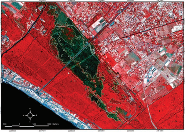
Fig. 6.10. Ikonos composite 124 image used for mapping burned pine forest ( P. pinea ) close to Rome after a fire event in 2000
