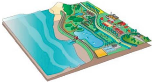
Fig. 3.12 Regulated tidal inlet (Source: Oedeckerk, 2006)
