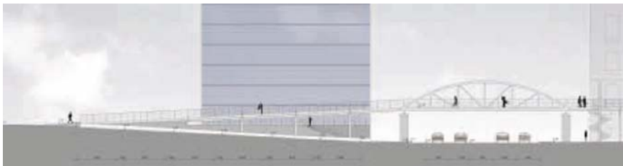
Fig. 3.37 A footbridge becomes an emergency and evacuation route (Source: GHS, 2002)
