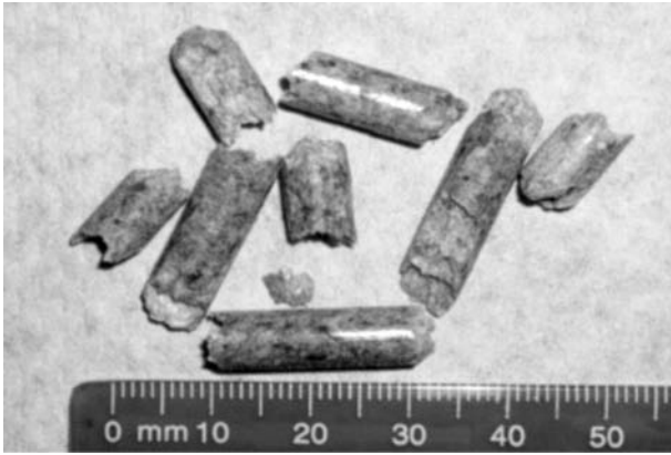
Figure 4.9. Picture of softwood pellets. Note: Ruler scale is in millimeters (Hartley and Wood, 2008; reproduced with permission from Elsevier).
