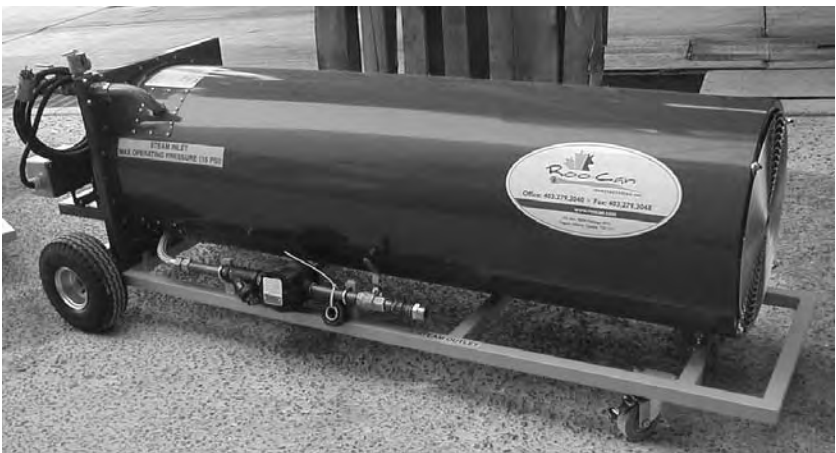
Fig. 8.14b. Portable low-pressure steam heater used in food-processing facilities.
