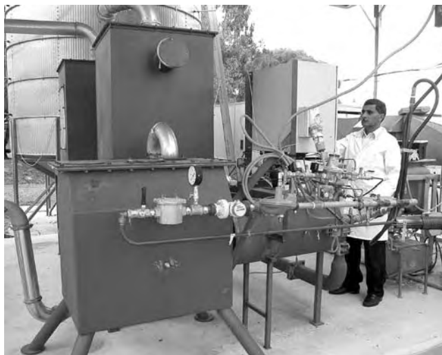
Fig. 8.10. Prototype of continuous-flow spouted bed heat disinfester (8 t/h capacity).
