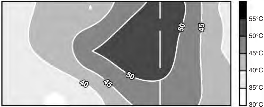
Fig. 8.13. Temperature gradients that develop during the heat treatment of a flour mill. The target temperature is 50–57°C for 24–36 h (from A.K. Dowdy, 1999, personal communication).
