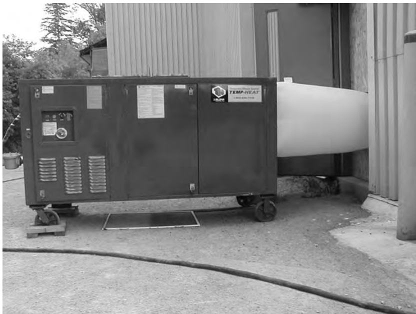
Fig. 8.14c. Propane-fired heater used in food-processing facilities.
