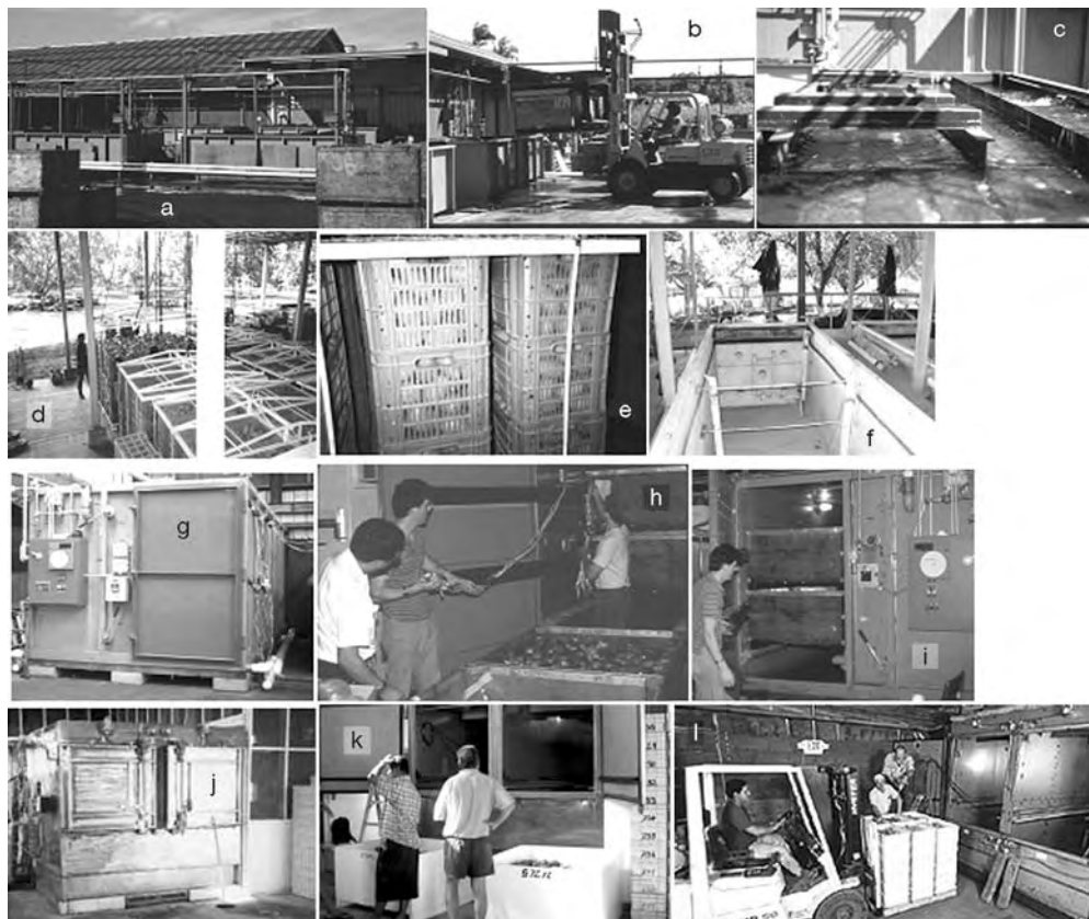
Fig. 13.6. Commercial heat treatment equipment: (a, b, c) Double hot water immersion treatment for papaya at AMFAC Tropical Fruits, Keaau, Hawaii, USA (c.1986) showing line of immersion tanks, forklift placing bin of papayas in tank and papayas held under heated water by wooden grate; (d, e, f) hot water immersion tanks for treating mangoes for export, Tapachula, Mexico, showing fruit being lowered into tank for treatment, bins of mangoes and empty treatment tank with water circulator openings at end; (g, h, i) a forced hot-air treatment unit at Tropical Hawaiian Products, Keaau, Hawaii (c.1989) showing operators preparing to insert temperature probes while a USDA-APHIS inspector watches, and preparing to close and lock chamber for treatment; (j, k) a double-wide, forced hot air and vapour heat treatment unit at Nature's Way Cooperative, Suva, Fiji, showing loading operations; and (l) loading double-wide, forced hot air and vapour heat treatment chamber at Dole Tropical Fruits, Kahuku, Hawaii.
