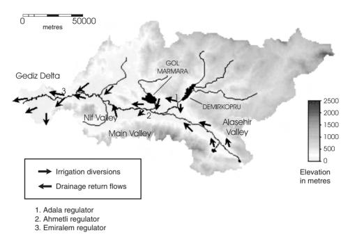
Fig. 11.2. Irrigation and drainage flow patterns, Gediz basin.
