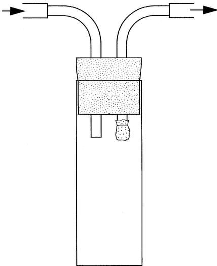
**Fig. 3.3** An aspirator for collecting rapid mites and relatively large mites, with arrows indicating the direction of air flow (D. Helmore).
