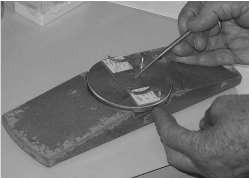
**Fig. 3.5** Turntable for sealing cover slips on glass slides using a brush and insulating paint or other sealants.
