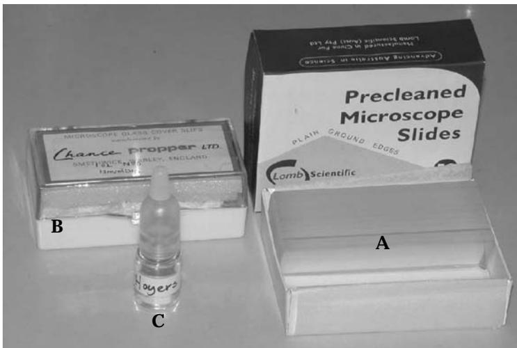
**Fig. 3.2** Some slide-mounting necessities. A, glass slides; B, round or square cover slips (box shown here); C, drop bottle for mounting media.
