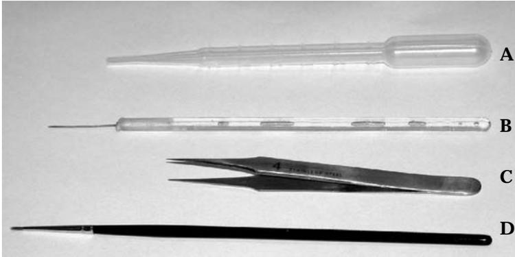
**Fig. 3.1** Some useful tools for collecting and preparing mites. A, pipette; B, pin mounted on a plastic stick; C, forceps; D, fine hair brush (size 000).
