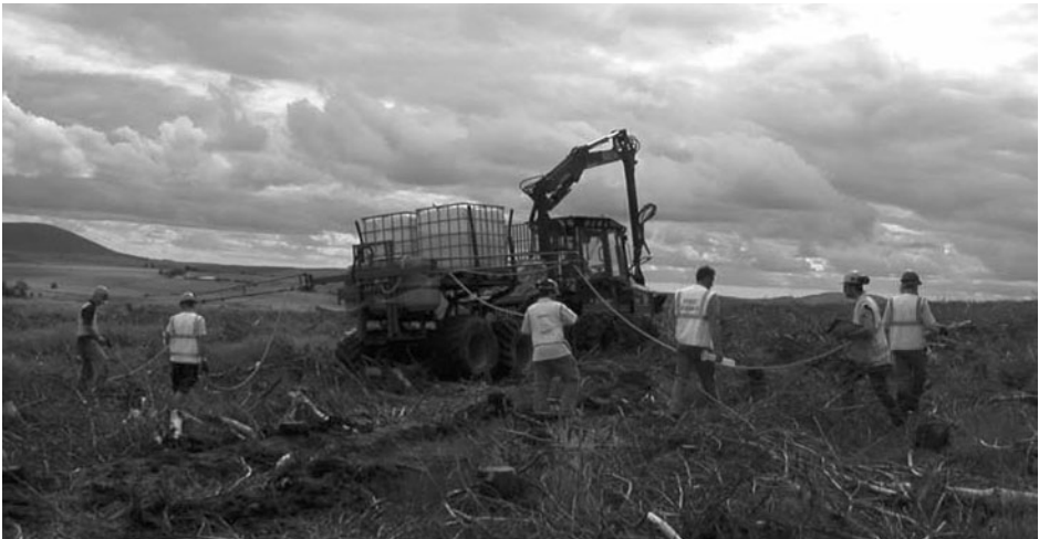
Fig. 15.6. Workers from Forest Research applying Steinernema carpocapsae at a clear-felled Sitka spruce plantation in Moray Firth, Scotland, using a forwarder-mounted spray rig fitted with bulk water tanks and four spray lances.
