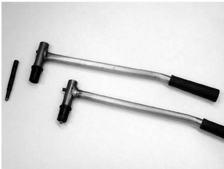
Fig. 21.6. Wad punch mounted in a hammer enables clean cutting of the tree's tracheids so that nematodes can enter.
