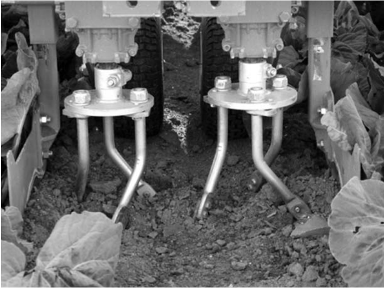
Fig. 8.8. Photo of the Weed-Fix cultivator, a vertical-axis rotary cultivator. (Photo by Wageningen UR Applied Plant Research.)
