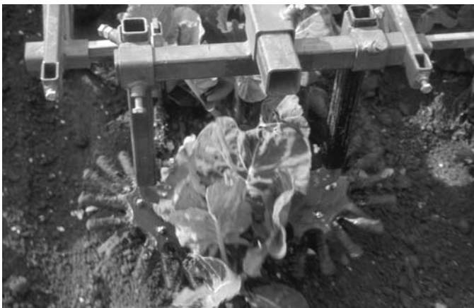
Fig. 8.10. Finger weeders, manufactured in Europe, operating in transplanted cabbages. (Photo by Wageningen UR Applied Plant Research.)
