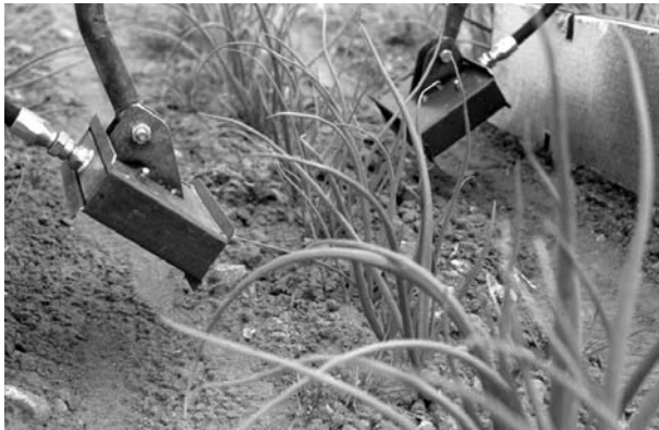
Fig. 10.3. Burner settings in selective flame weeding in onions. (Photo by Johan Ascard.)
