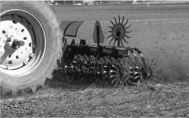
Fig. 8.6. Rotary hoe in action in cereals. (Photo by Maryse Leblanc.)
