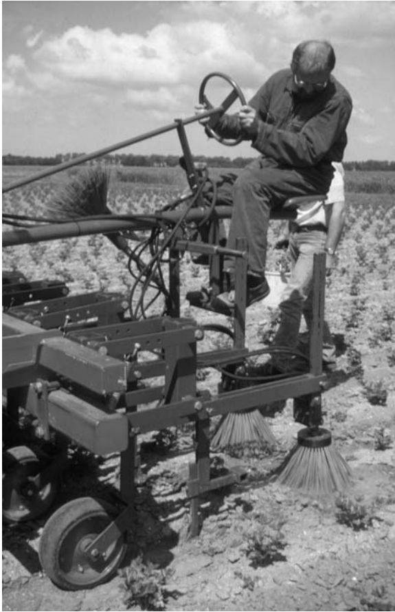
Fig. 8.7. Vertical axis brush weeder. (Photo by Wageningen UR Applied Plant Research.)
