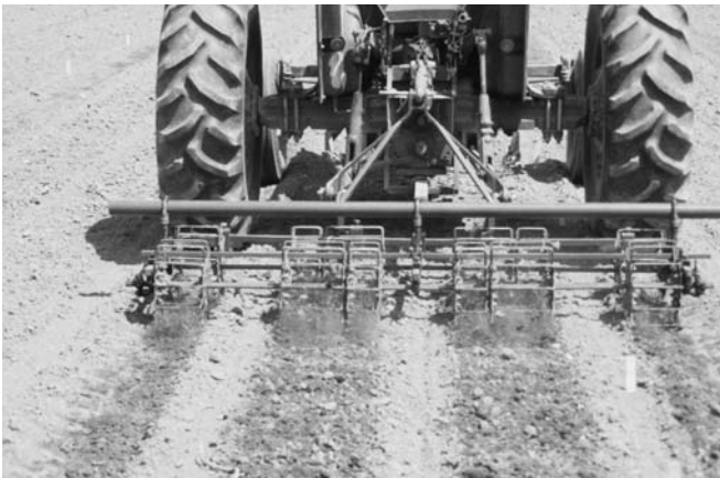
Fig. 8.9. Photo of the Budding basket weeder Model K used in carrots. (Photo by Daniel Cloutier.)
