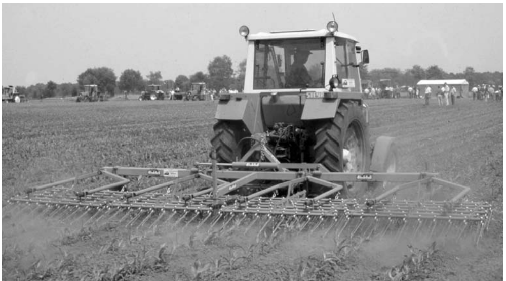
Fig. 8.4. Flex-tine harrow in silage maize. (Photo by Wageningen UR Applied Plant Research.)
