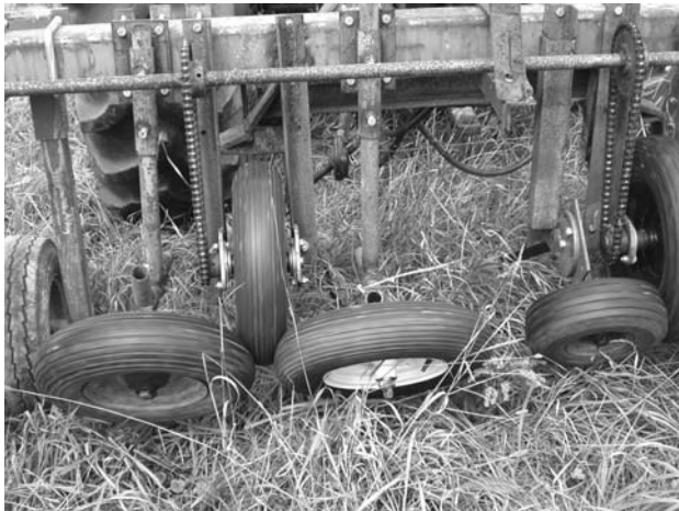
Fig. 8.17. Weed puller developed to pull wild mustard from soybean fields in south-western Quebec. (Photo by Daniel Cloutier.)
