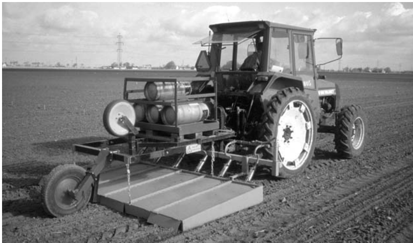
Fig. 10.5. Non-selective flame weeding pre-emergence of the sugarbeet crop using a Swedish flamer with one burner per row and one common insulated cover. (Photo by Johan Ascard.)
