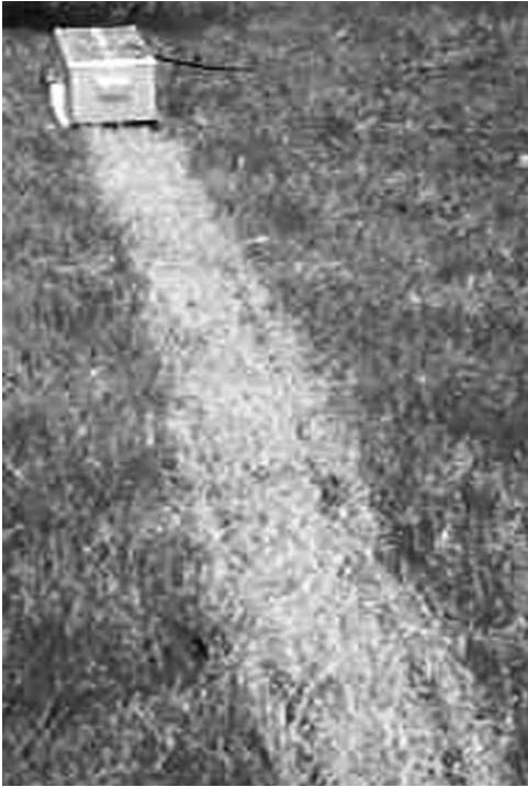
Fig. 10.14. Experimental UV application equipment. Demonstration of the instantaneous effect on grass. Regrowth can be a problem (see http://www.kaj.dk/weed-by-uv.htm ; Kaj Jensen's homepage).
