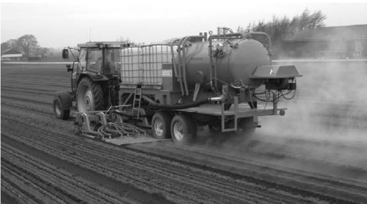
Fig. 10.11. Band steaming for weed control and partial soil sterilization before sowing of sugarbeets. This nine-row band steamer, built by a Swedish farmer, has a capacity of 1 ha per 8 h and requires 690 l/ha of diesel fuel to obtain a 95% reduction in weed emergence. (Photo by Johan Ascard.)
