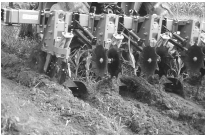
Fig. 8.15. Ridging in maize utilizing special wings mounted on an inter-row cultivator. (Photo by Daniel Cloutier.)
