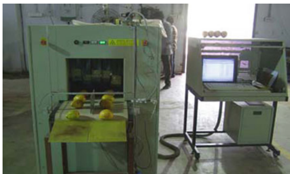
Fig. 5.8 X-ray based sorting system for mangoes (Courtesy: CEERI, Chennai, India)
