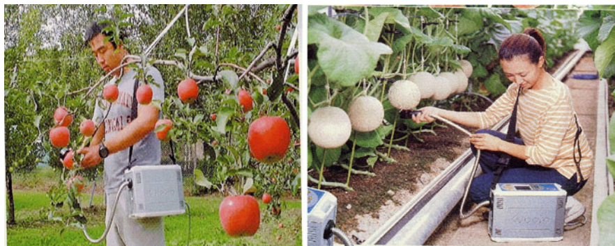
Fig. 6.33 NIR based fruit tester being used for checking the maturity of apple and muskmelon
