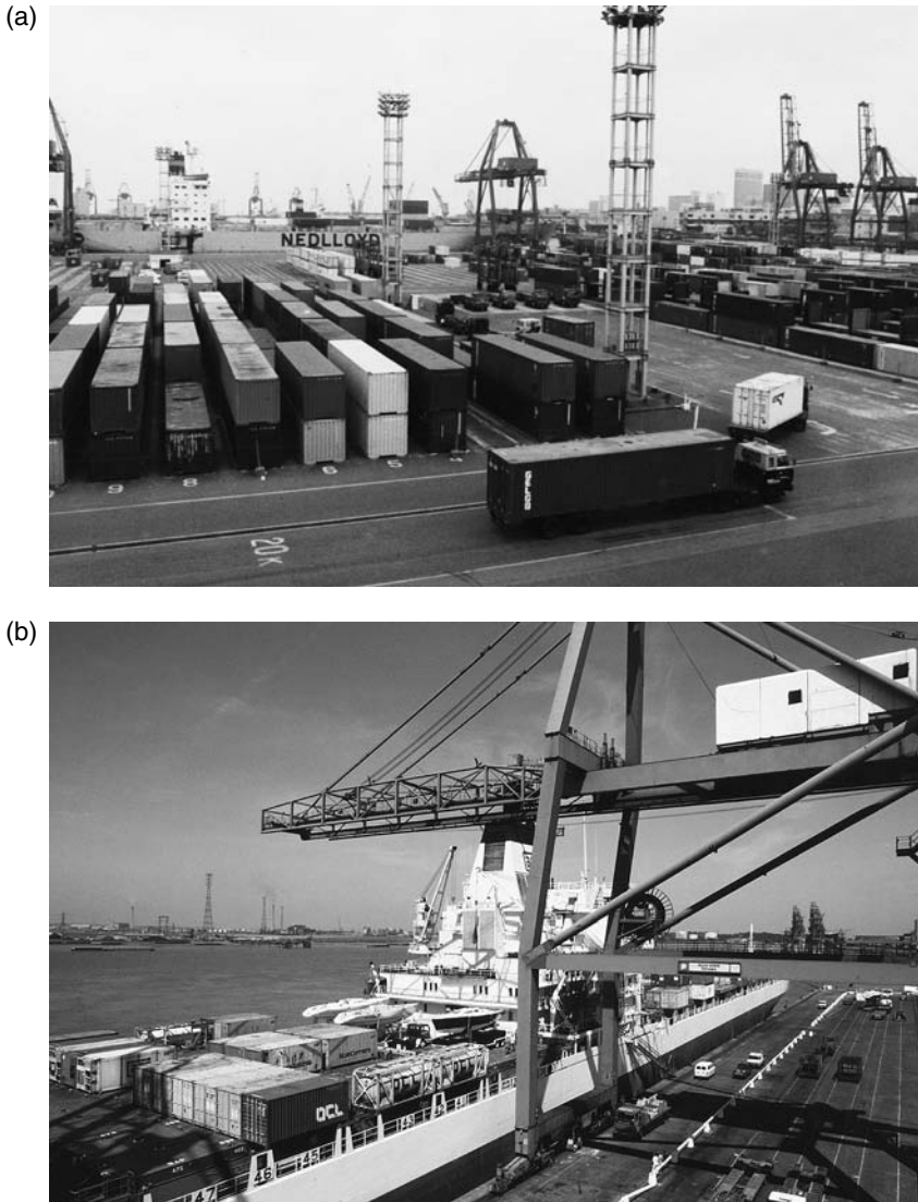
Fig. 1.2. Container transport by land and sea. (a) Delivery of containers to a large container terminal by truck. (b) A specialized container gantry loading containers on to a container ship. (Photo courtesy of PHSI, Defra. Crown copyright.)
