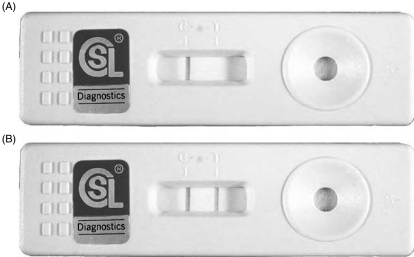
Fig. 10.5. Lateral flow device for serological diagnosis of viruses and other pests: (A) negative; (B) positive. (Courtesy of CSL. Crown copyright.)
