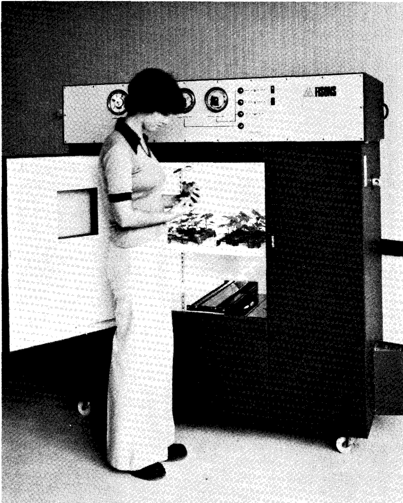
Fig. 1-4 A controlled-environment cabinet in which small plants can be grown at a constant temperature. (Photograph reproduced by kind permission of Fisons Scientific Apparatus Ltd, Loughborough, Leicestershire.)
