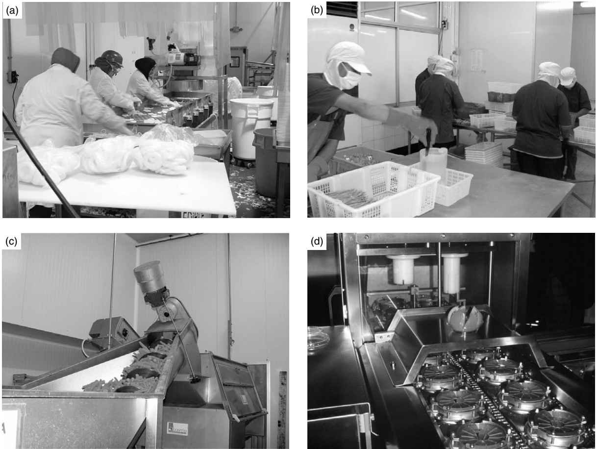
Figure 10.6 (a) slicing onions; (b) trimming asparagus; (c) peeling carrots; (d) slicing tomatoes in fresh-cut processing plants.
