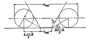
FIG. 3. Calculation of diameter at small end of cone.
