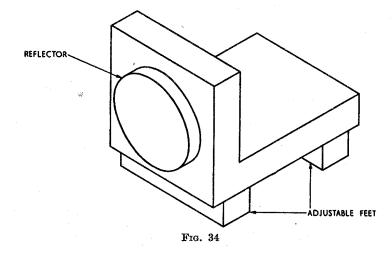
may be a lapped and polished surface of the block itself. If of glass, it should be coated with reflecting material, generally aluminium or rhodium, on its front face, not on the back.
