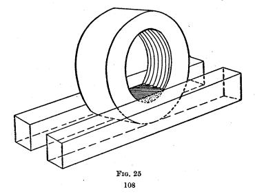
when an internal effective diameter machine is not available. A cast of an internal thread must be made before the form and angle can be measured, and this experiment is mainly directed towards the method of taking the cast.
