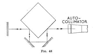
seen that *nine* reflections are involved. It is true that the sensitivity of the auto-collimator is doubled, but this advantage can easily be offset by the poor quality of the image. Setting up needs great care and much patience. The reflectors must be accurately placed and their full apertures must be utilised. Only good surface reflectors will give any image at all; the best are probably aluminised or rhodiumised glass.
