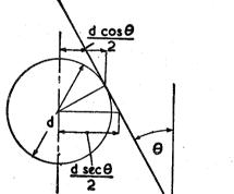
FIG. 4. Taper Plug Gauge measured with rollers, with geometry of roller contact.
