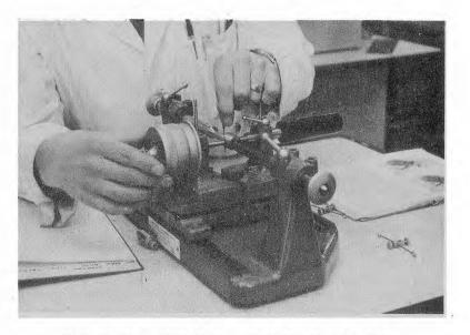
Plate 1. A Floating Micrometer Measuring Machine See Experiment 19
