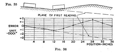
This first reading represents the angular direction of the first span of the carriage. If the edge were perfectly straight, the same reading would be obtained wherever the carriage was placed along the straightedge. Any errors from true straightness will be shown as angular variations at various positions.
