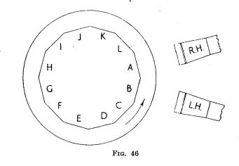
Before starting the calibration the direction of sign of the measuring auto-collimator must be determined. This can be done by setting the measuring auto-collimator to read on one of the faces and giving the table a slight *clockwise* rotation. Such a rotation would correspond to an *increase* of the subtended angle (or the angle of rotation) between two adjacent faces. The direction of auto-collimator reading for this rotation should be carefully noted and, if possible, the auto-
