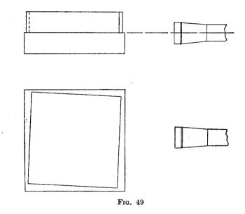
The images can be identified by masking one face at a time. It will also be assumed that the auto-collimator gives an increasing reading for a clockwise rotation; this is true for the Microptic instrument in its normal position for horizontal reading.
