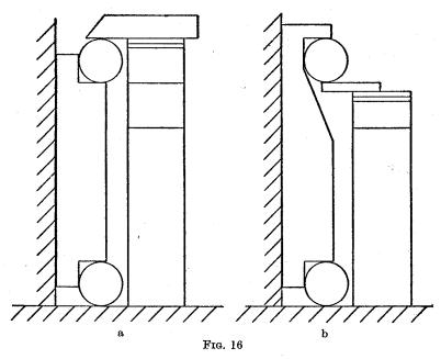
(1) Equality and uniformity of diameter of rollers. It should be possible, with a bar of type (a), to compare the rollers on the comparator, using a suitable size of slip gauge as a measuring anvil and holding the bar so that a diameter lying at about  $45^{\circ}$  to the horizontal can be measured.
