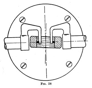
located in the same thread groove and a reading is obtained in the measuring head. Clamp the measuring head and the tailstock, remembering that there are several clamps to tighten. It is as well to go over this twice and work out a fixed routine for tightening the clamps. One loose clamp is sufficient to spoil the entire experiment.
