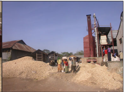
Recirculating dryer fuelled by shelled maize cobs.
