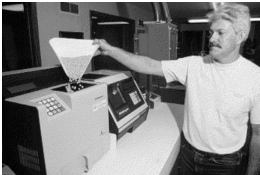
FIGURE 9.3. NIR spectrometer measurement at elevator facilities
