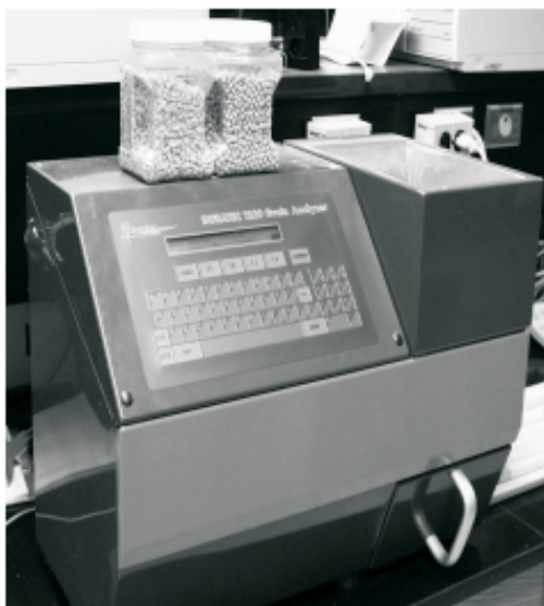
FIGURE 9.7 Officially approved NIR spectrometer for grain analyses in the United States: FOSS Tecator Infratec 1229 Grain Analyser
