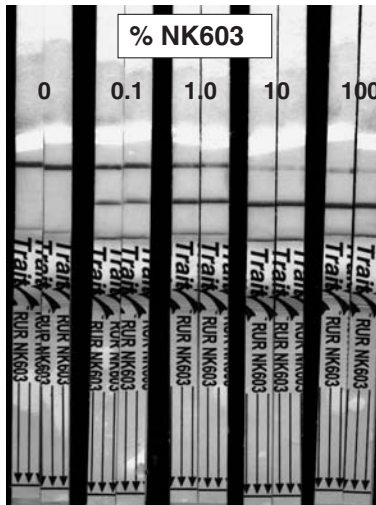
FIGURE 6.9. Sensitivity of strip-test method for RR corn event NK603 expressing CP4 EPSPS
