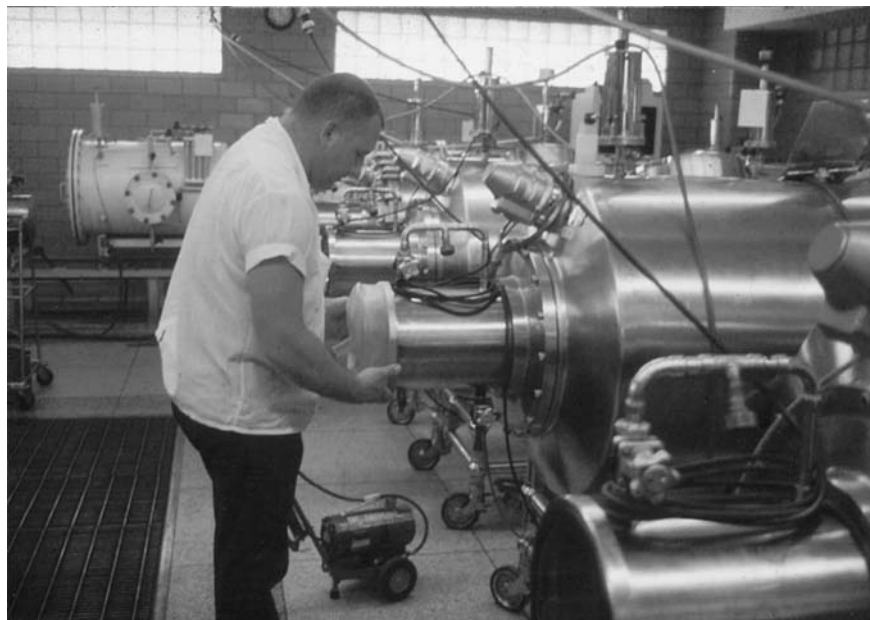
FIGURE 46.2 Steel isolator with entry port capped with plastic in preparation for chemical sterilization of materials.
