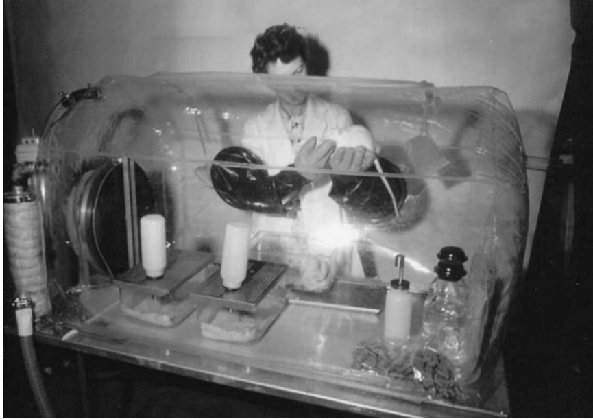
FIGURE 46.3 Plastic isolator with air filter in foreground and outlet trap partially visible behind the filter.
