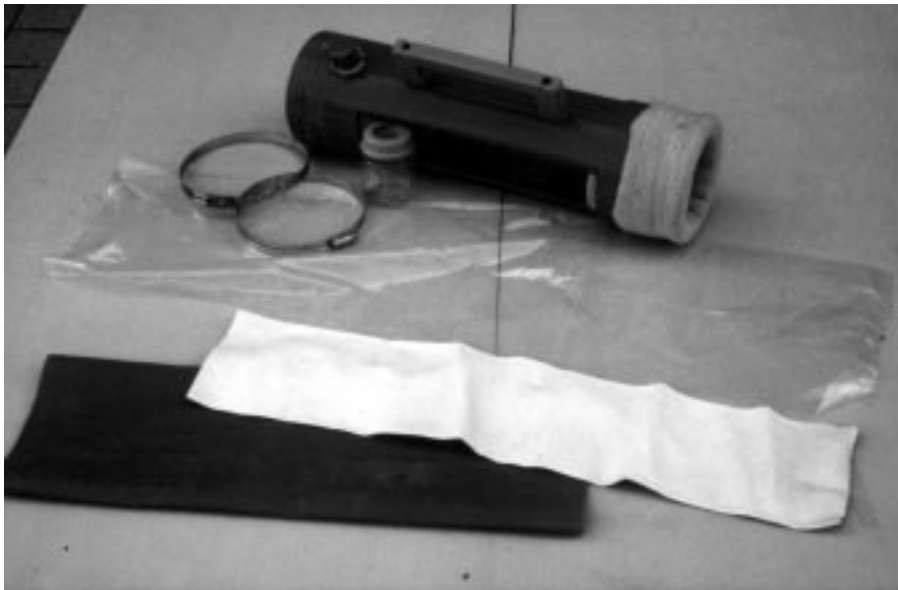
Fig. 5.3. A dismantled Cambridge AV, illustrating the component parts including the outer and inner linings.
