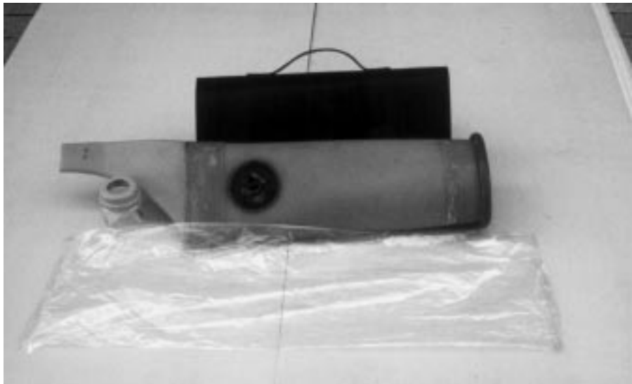
Fig. 5.7. The dismantled Missouri AV, illustrating the component parts and the liner used.
