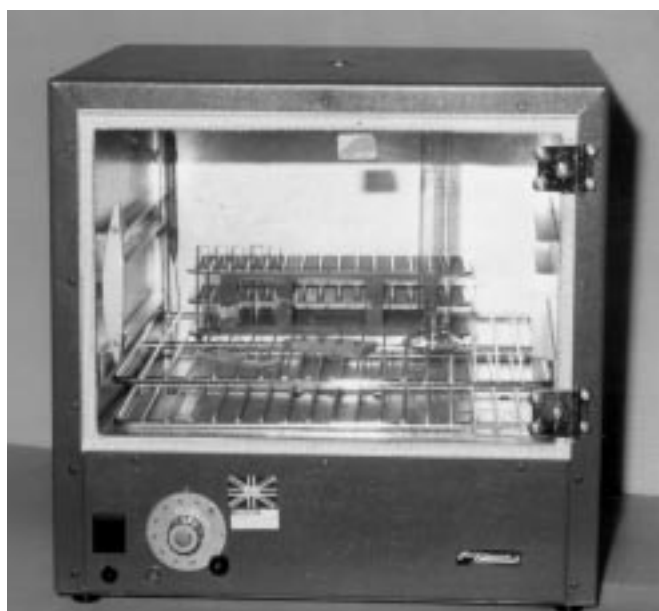
Fig. 6.1. A small portable incubator is particularly useful for the storage of glassware and semen during the evaluation process.
