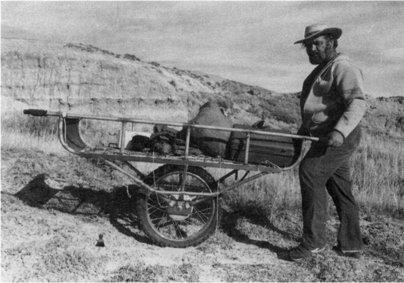
Bob Makela with one of his field inventions, the Dino Wheel, which can be used by two people to get heavy loads in and out of areas having no roads. ( Pat Leiggi, reproduced courtesy of the Museum of the Rockies. )
