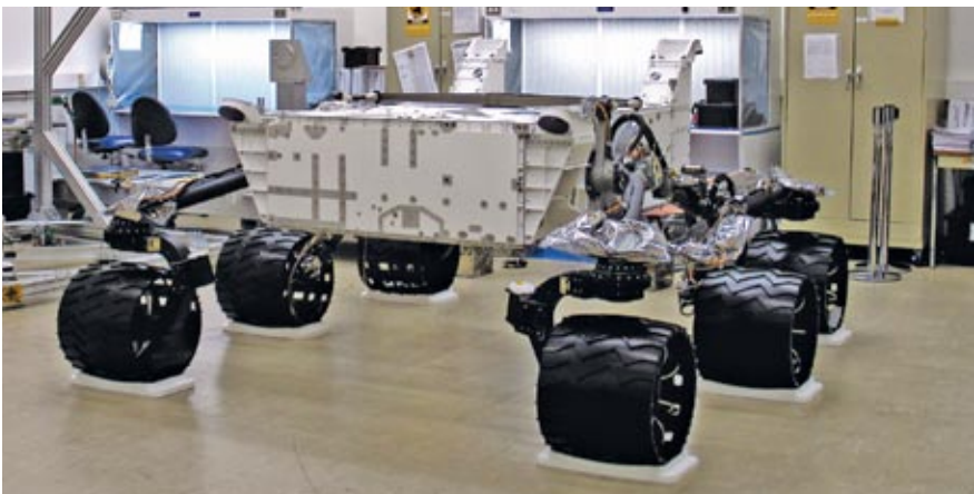
PRICEY PROBLEMS: Mars Science Laboratory rover has had troubles with actuator motors for its wheels and other systems. Fixing them is one reason project costs have skyrocketed.
