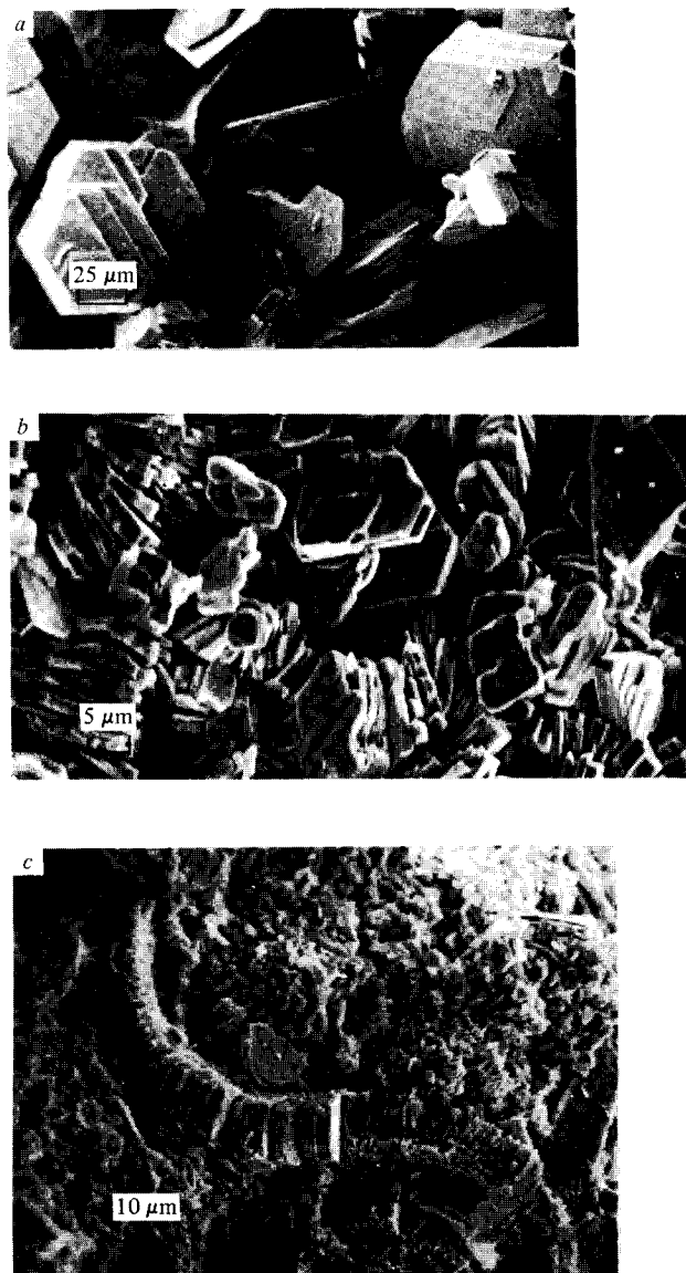
Figure 6.29. Scanning electron micrographs of kaolinite minerals. (From Keller & Hanson, 1975, and Keller, 1976, 1977.) (a) Dickite from Anglesey, Wales. (b) Kaolinite from Keokuk, Iowa. (c) S-shaped 'book' or 'vermiform' of kaolinite from Hodges mine, Georgia Kaolin Co. (d) Grooved vermiforms of kaolinite from Jacal, Mexico. (e) Kaolinite vermiforms and books showing complex grooving.
