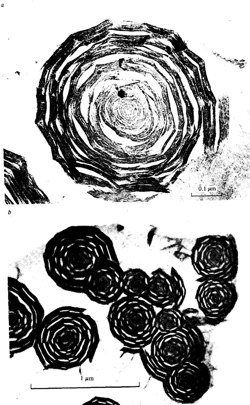
Figure 6.33. (a) and (b) Transmission electron micrographs of spiral discs of halloysite from Pahoia Tuff, New Zealand. (From Kirkman, 1977.)
