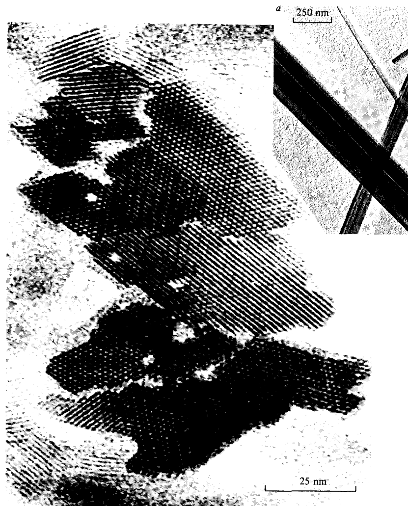
Figure 6.48. Electron micrographs of sepiolite (from Rautureau & Tchoubar, 1976). (a) Grooved sepiolite laths. (b) Cross-section at high magnification showing channels in the crystal structure (cf. figure 6.47) as well as larger holes running through the crystal.
