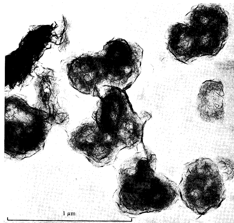
Figure 6.56. Synthetic hectorite. Transmission electron micrograph showing partly transformed brucite crystals, 'doughnuts', enclosed in hectorite 'bags'. (From MacKenzie, 1971.) This stage was reached after 6 days reflux of a slurry of composition \text{SiO}_2:\text{MgO}:\text{LiF} = 0.01:1.0:0.25 in pyrex glass.
