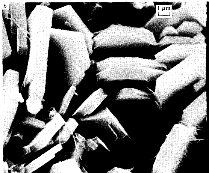
Figure 6.26. Scanning electron micrographs of zeolites in sedimentary rocks. (From Mumpton & Ormsby, 1976.) (a) Analcrite blocks. (b) Clinoptilolite plates with a few threads of mordenite. (c) Erionite bundles. (d) A 'rat's nest' of interlaced mordenite fibres.
