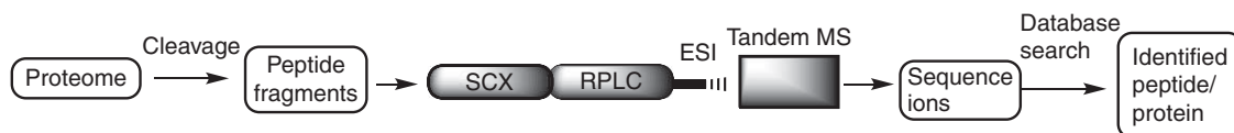
Figure 4 Depiction of shotgun proteomics using multidimensional protein identification technology; a complex mixture of peptide fragments in the digest are resolved by a combination of ion-exchange and reversed-phase liquid chromatography.
