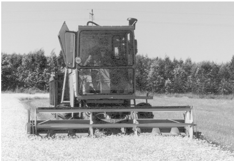
FIGURE 5.9.3 Chamomile harvester (Argentine type).
