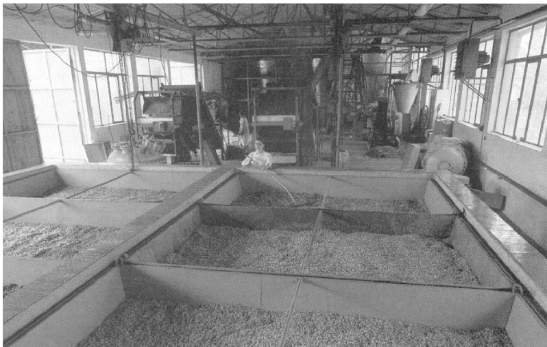
FIGURE 8.2.7 Static dryer for chamomile in Slovakian Republic.
