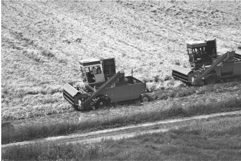
FIGURE 5.11.2 Chamomile harvest with the Linz III picking machine.
