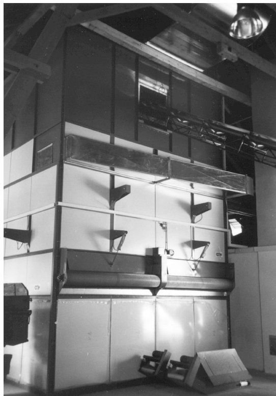
FIGURE 8.2.9 Basculating tier dryer (kiln) [3, 4].
