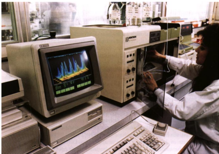
Figure 11. High Performance Liquid Chromatography apparatus with supporting equipment.
