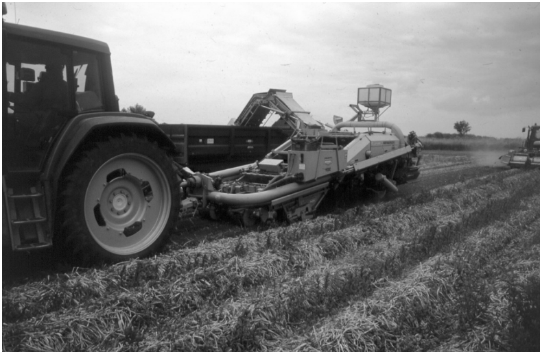
Figure 4.8 Large unmanned bulb lifter discharging into bulk trailer (Photograph: Horticulture Research International).
