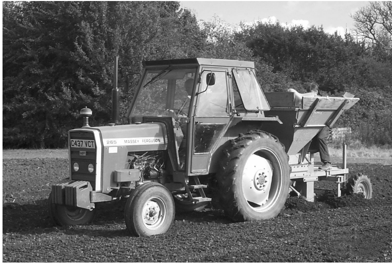
Figure 4.4 A typical bulb planting machine feeding bulbs from a hopper into two ridges (Photograph: Horticulture Research International).
