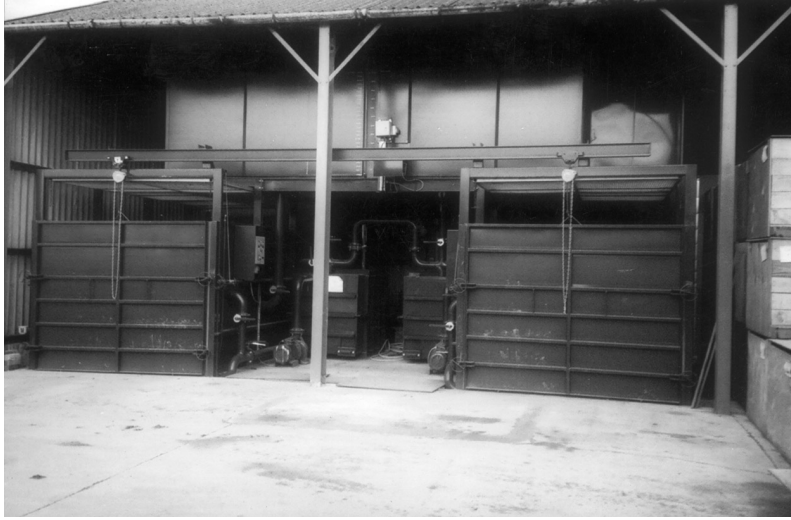
Figure 4.3 Modern front-loading hot-water treatment tanks. Two four-tonne units with overhead slave tank for holding dip when loading and unloading bulbs (Photograph: Lyn Secker, Secker Welding, Holbeach).
