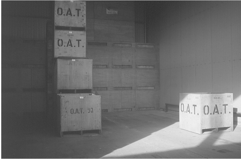
Figure 4.9 Letter box drying wall for bulbs in bulk bins. Air is blown through the slots in the wall into the pallet bases of the one tonne bins which are stacked against them (Photograph: Horticulture Research International).
