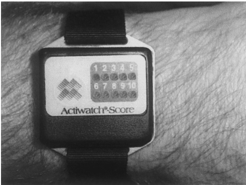
Figure 10.10 Close up view of the ActiWatch-Score device that is used to monitor sleep/wake activity and provide a means for the subjects to enter data about their drinking behavior in real time.
