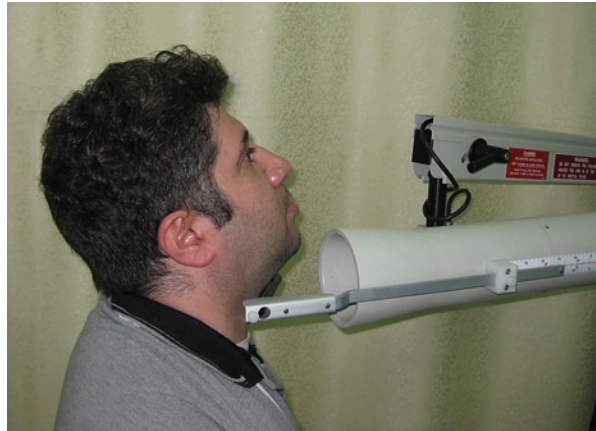
Fig. 4.7 Thyroid probe for radioiodine uptake study
