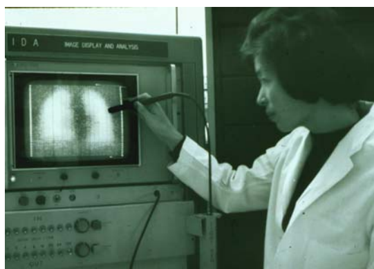
Figures 66 and 67 First use of a mini-computer (IDA) to quantify regional perfusion of the lungs in 1968.
