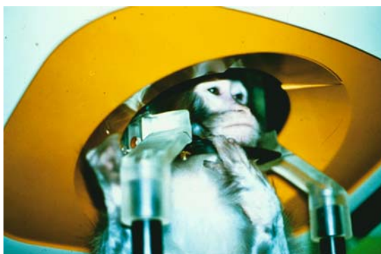
Figure 176 PET scanner designed by Hamamatsu Photonics for the study of unanesthetized monkeys.
