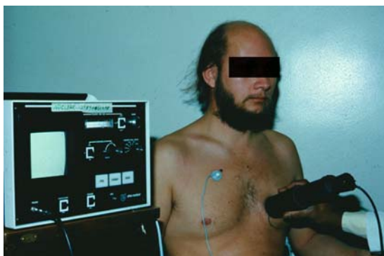
Figure 150 The “nuclear stethoscope” invented at Hopkins to examine the movement of blood through the chambers of the heart.
