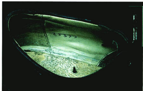
Fig. 3.2 Nail has penetrated the sole of the shoe—the insole has been removed to reveal the nail.
