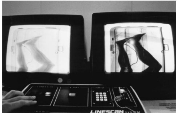
FIGURE 26.3 Linescan fluoroscope used for baggage inspection is useful for preliminary inspection through body bags or caskets. Pertinent anatomic lesions, foreign bodies, and ordnance can be found.
