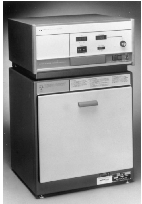
FIGURE 18.21 Desktop model, Faxitron X-ray Unit. The controls are on top. The cabinet below contains the specimen and the film.
