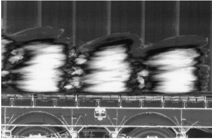
FIGURE 30.8 Liquid in containers inside a truck makes a wavy pattern as it sloshes around. This is illegal alcohol being hauled in a truck supposedly loaded with solid freight.
