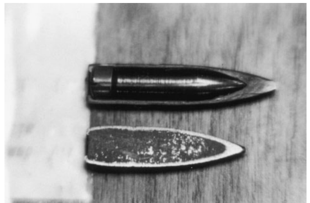
FIGURE 17.18 Above is a cross section of a military hardcore projectile. Below is the cross section of an ordinary military projectile with a complete steel coat or jacket.
