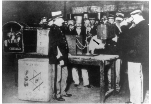
FIGURE VII.I The French customs officer on the right uses a handheld fluoroscope to examine a piece of luggage held between the fluoroscope and a naked x-ray tube (arrow). (From Angus, W.M., RadioGraphics , 9, 1225, 1989. With permission.)
