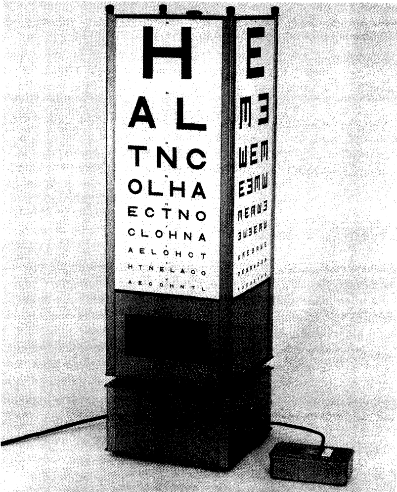
Fig. 5.2 Snellen distance test type. Also shows a duochrome test below and an 'E' test chart.
