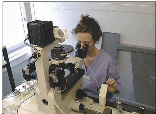
Micromanipulation equipment required to undertake ICSI procedures. The embryologist guides the needle into the egg using joystick directed servomotors
