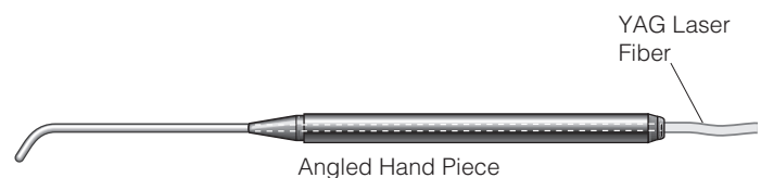
Figure 5 Shown is an angled handpiece through which an yttrium-aluminum-garnet (YAG) laser can be placed during VATS. The handpiece is narrow enough to be used during thoracoscopy as well as during open procedures.
