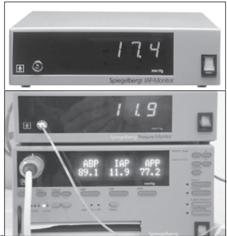
Figure 42. Combination of the Spiegelberg IAP and APP monitor allowing continuous fully automated monitoring. IAP: intra-abdominal pressure; ABP: arterial blood pressure; APP: abdominal perfusion pressure.
