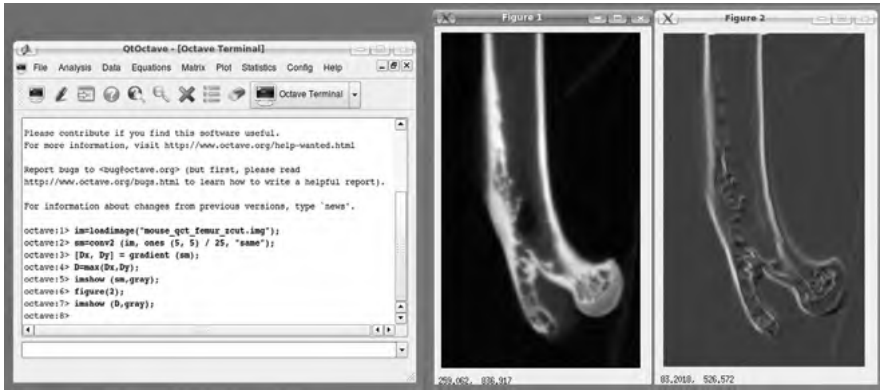
FIGURE 14.2 Image processing with a scripting language, in this example with Octave. The screenshot shows QtOctave, a graphical environment for Octave, and two images that were generated with a few commands. The commands can be seen in the QtOctave window and perform the following steps: (1) load an image file and store in the variable im ; (2) convolve the image with a 5 \times 5 matrix of 1/25 (box smoothing filter) and store the result in sm ; (3) compute the gradients in the x and y directions; (4) take the maximum of the gradients in the x and y directions to approximate Sobel-like behavior; (5) display the smoothed image sm ; (6) and (7) display the gradient image D in a new window.
