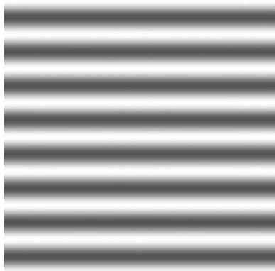
FIGURE 3.4 Demonstration of Fourier-based filtering. After removal of the peaks on the u -axis in Figure 3.3B and inverse Fourier transform, only the oscillations along the y -axis remain.
