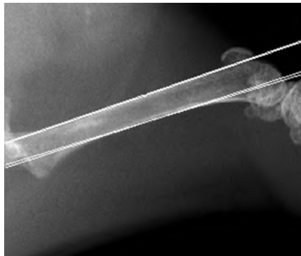
FIGURE 7.6 The inverse Hough transform of the local maxima in Figure 7.5 superimposed on the original x-ray image. The local maximum for the lower edge was ambiguous (two pixels of an identical number of votes), and two closely aligned lines emerge.
