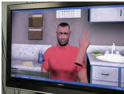
FIGURE 13.13 Training of medical students with a virtual patient. The setting is an ophthalmologist's office, and the patient can be asked to perform various tasks, such as telling the number of fingers indicated, or following the hand with his eyes. In this simulation, the hand is controlled by the medical student by means of a three-dimensional positioning device. Simple clicks make it possible to extend a specific number of fingers. (Courtesy of Dr. Kyle Johnsen.)
