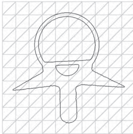
FIGURE 6.11 Edge image of a CT slice of a spine phantom with a grid of triangular cells superimposed.
