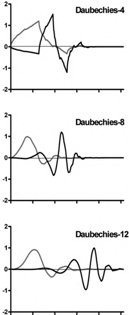
FIGURE 4.3 Some wavelets (black) and their corresponding scaling functions (gray) of the Daubechies family.
