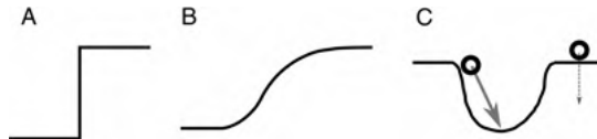
FIGURE 6.1 Sketch of an image edge (A) causing an external energy. The edge is shown in cross section (A). After Gaussian blurring (B) the edge is spread out. Its negative gradient (C) forms a canyon that attracts the snake by gravity. If the snake is near enough to the canyon walls, a strong external force exists (gray arrow) that pulls the snake toward the canyon bottom to lower its potential energy. Outside the canyon, however, the snake experiences no external forces (thin dashed arrow).
