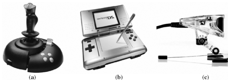
Fig. 1. Control devices: (a) Microsoft Sidewinder Force Feedback Joystick, (b) Nintendo DS Touchscreen, (c) TrackIR3 Pro
